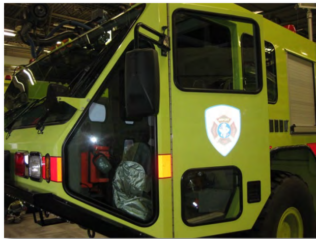
Figure 2-19 – Oshkosh 3000 Striker Vehicle at FAI. One person can drive the vehicle and simultaneously operate multiple fire suppression devices located on the outside of the vehicle.
