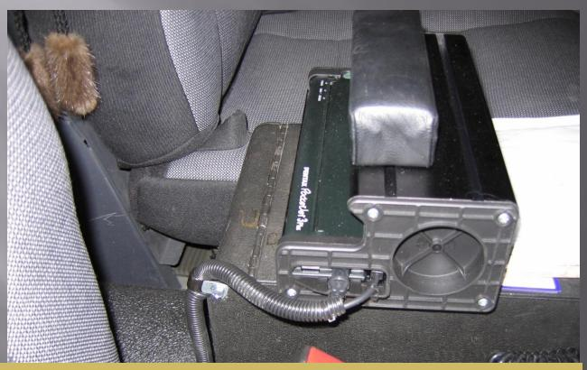
The Printer will be mounted in this location for most typical installations. We must be able to free up the area on the rear of the console to facilitate this type of mount. Some installations will require the removal of cup holders or storage pockets on the console.
