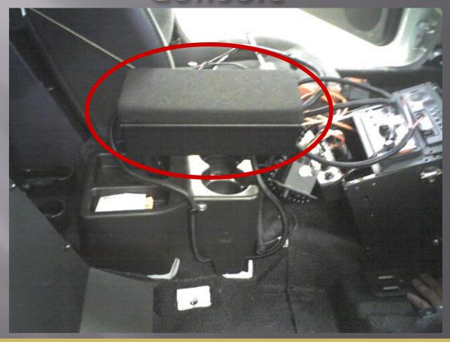
The Printer in most newer Impalas will be mounted in this location and can be swiveled to the side and tilted back for access to the OE Console
