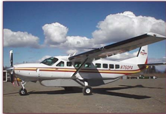
Figure 3-15 Cessna Caravan 208 with Belly Pod for Added Cargo
