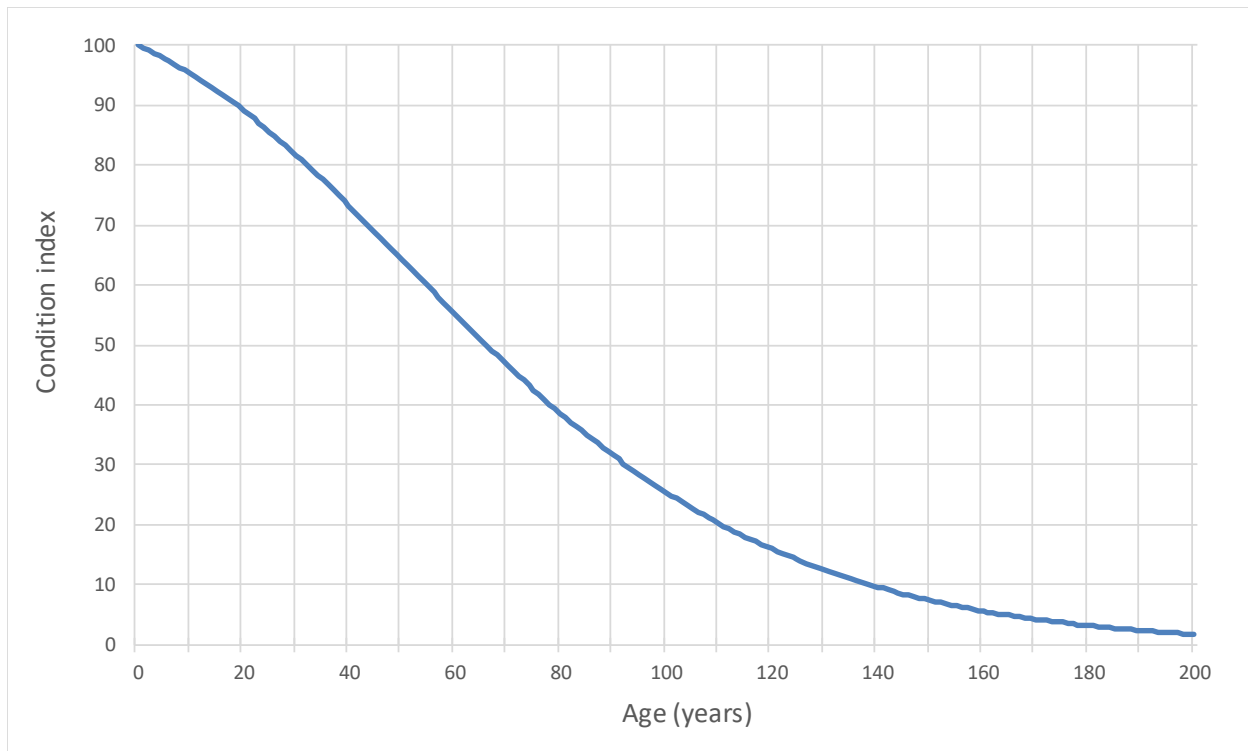
Figure 7-5: Deterioration of a typical maintenance station material site inventory due to material depletion
