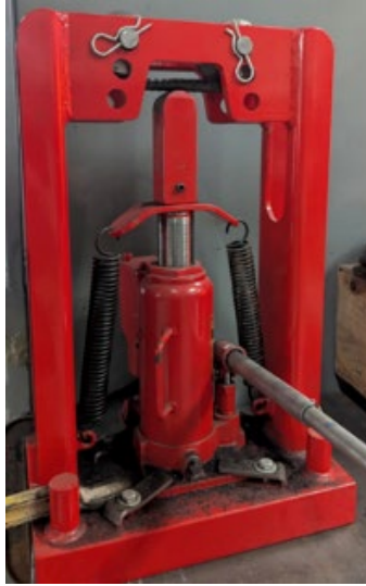
Figure 6: Test configuration for top-ejecting guided-bend test with lap-splice weld loaded.
