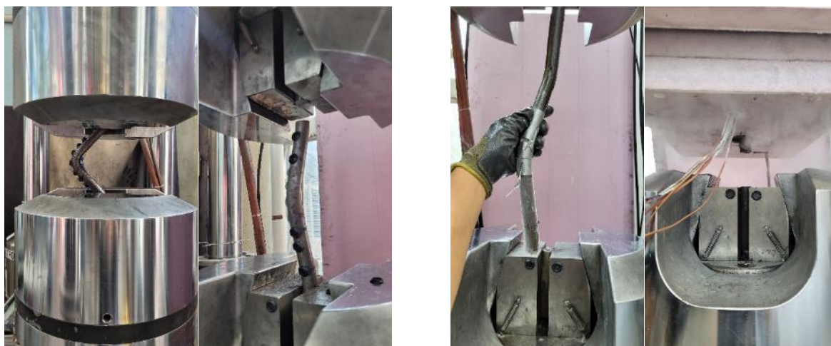
Figure 4-26 MA Smooth broken specimens with brittle failures, tested at room (a) and low (b) temperatures.
