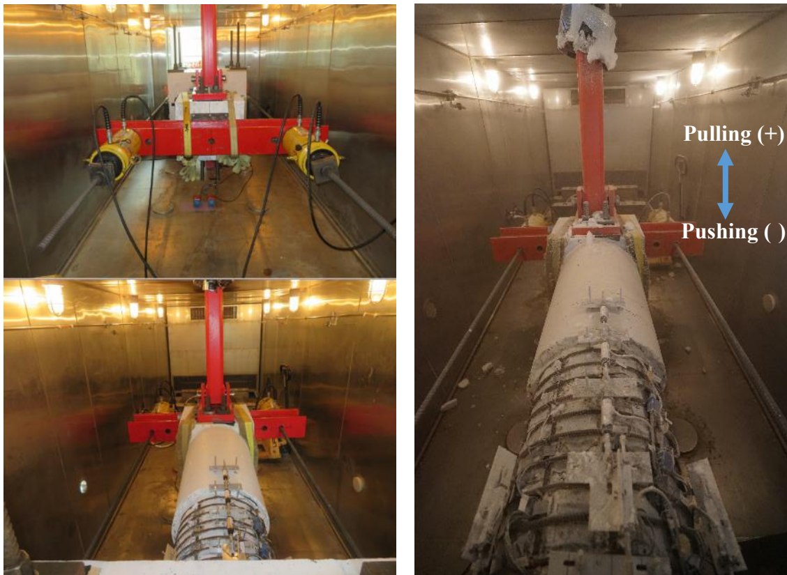
Figure 5-59 Experimental setup of the low-temperature quasistatic lateral cyclic column test
