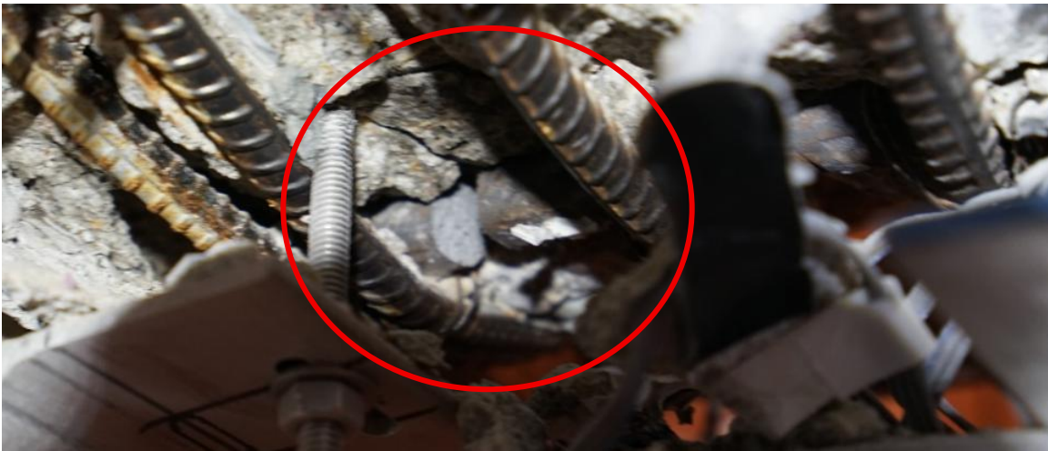
Figure 5-67 Second cycle of \mu 6 (pulling). Fracture the bottom extreme bar 2B
