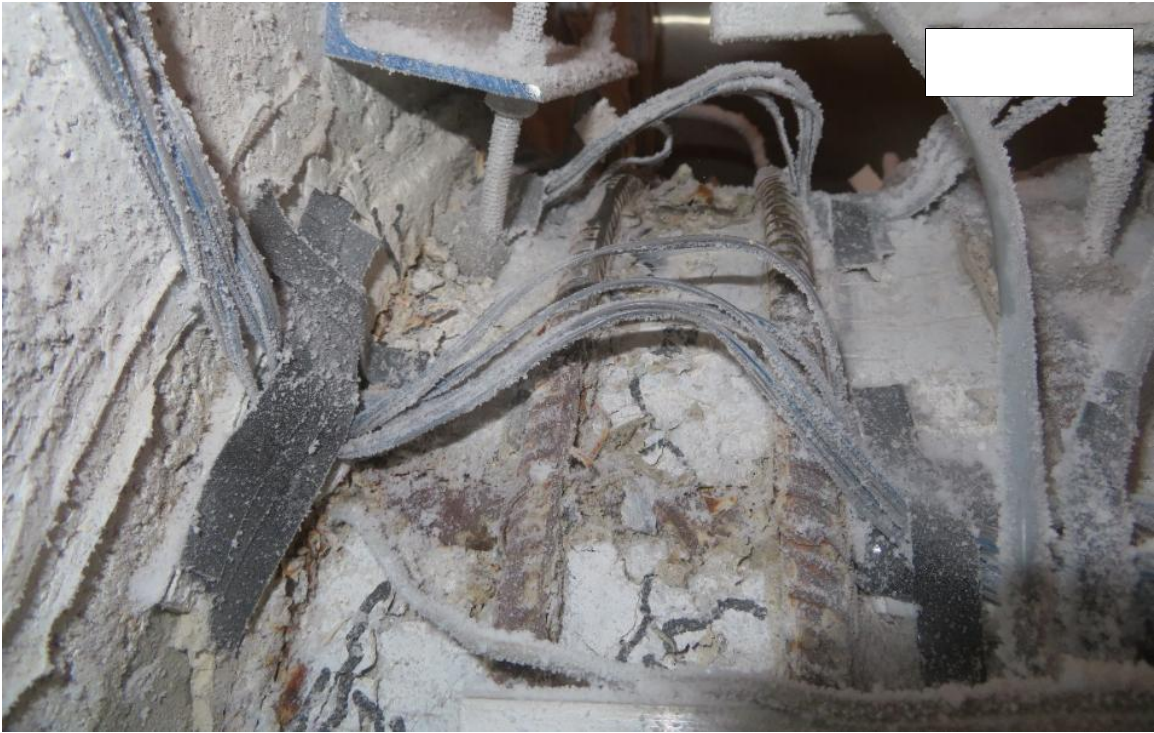
Figure 5-81 First cycle of \mu_4 (pulling): Concrete crushing
