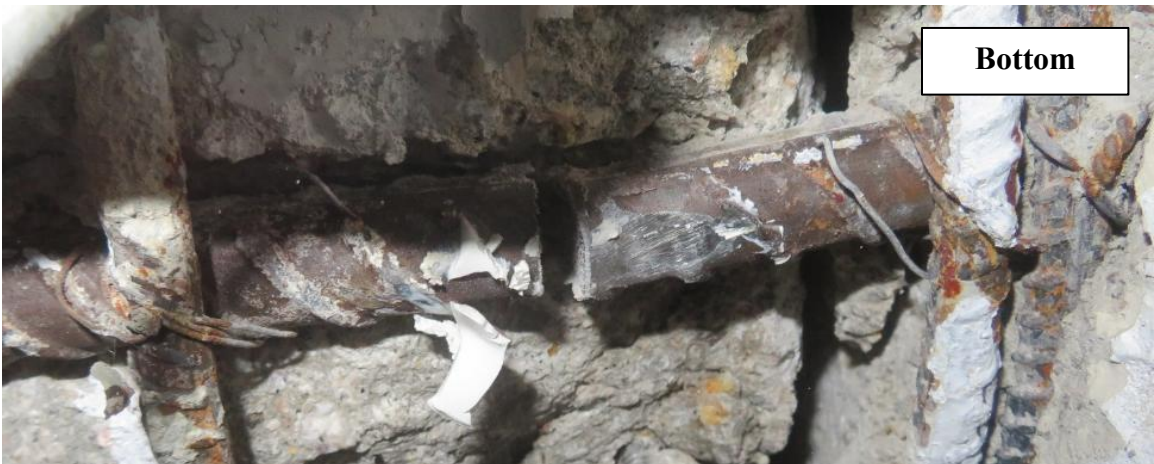
Figure 5-120 Second pulling cycle of \mu 5 : Bar fracture of adjacent bar to top extreme bar 1B
