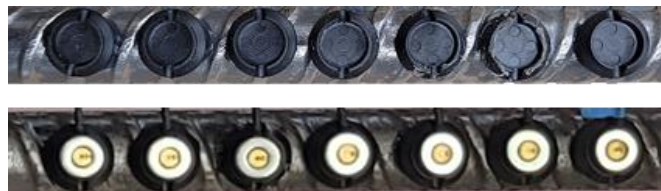
Figure 4-6 LED caps (top) and markers (bottom) on a reinforcing steel specimen.
