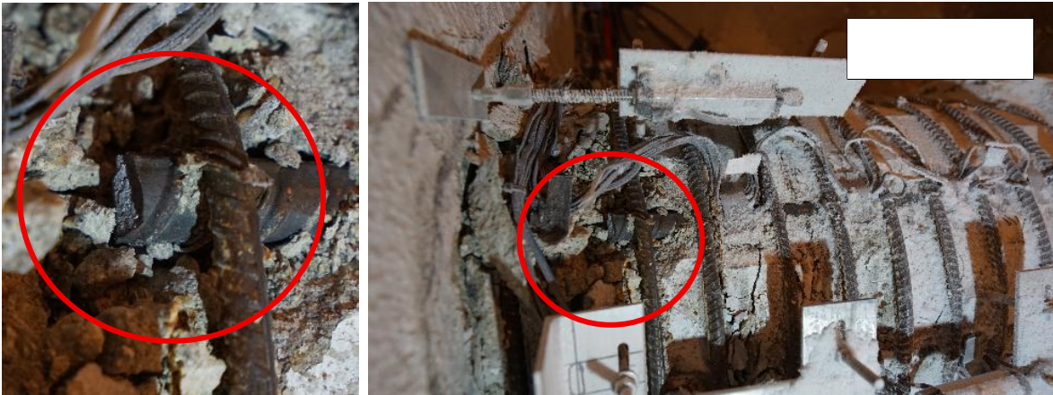
Figure 5-66 First pushing cycle of \mu 6 , fracture of top bar T1
