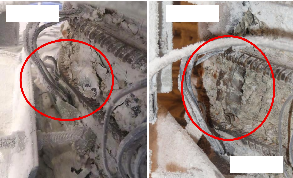
Figure 5-82 Spiral yielding in the third pulling cycle of \mu_4 and visible bar buckling in the first pulling cycle of \mu_5 – Top extreme bar 2B
