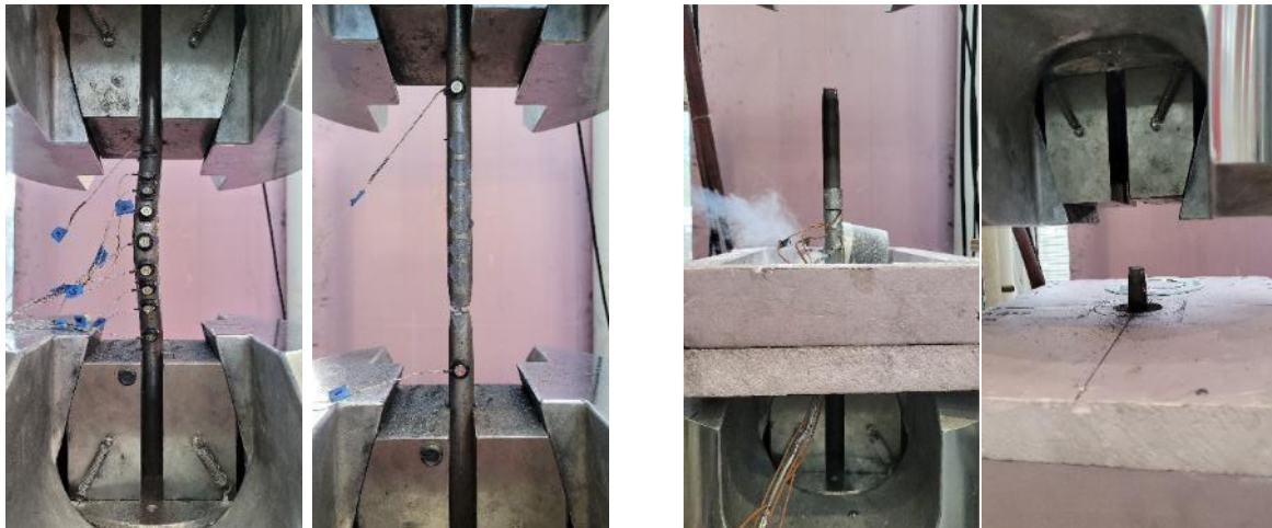
Figure 4-25 MA Smooth broken specimens with ductile failures, tested at room (a) and low (b) temperatures.
