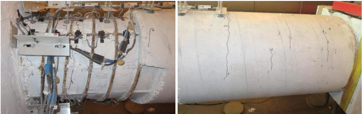
Figure 5-113 Third pushing cycle of \mu_1 : Extension of cracks
