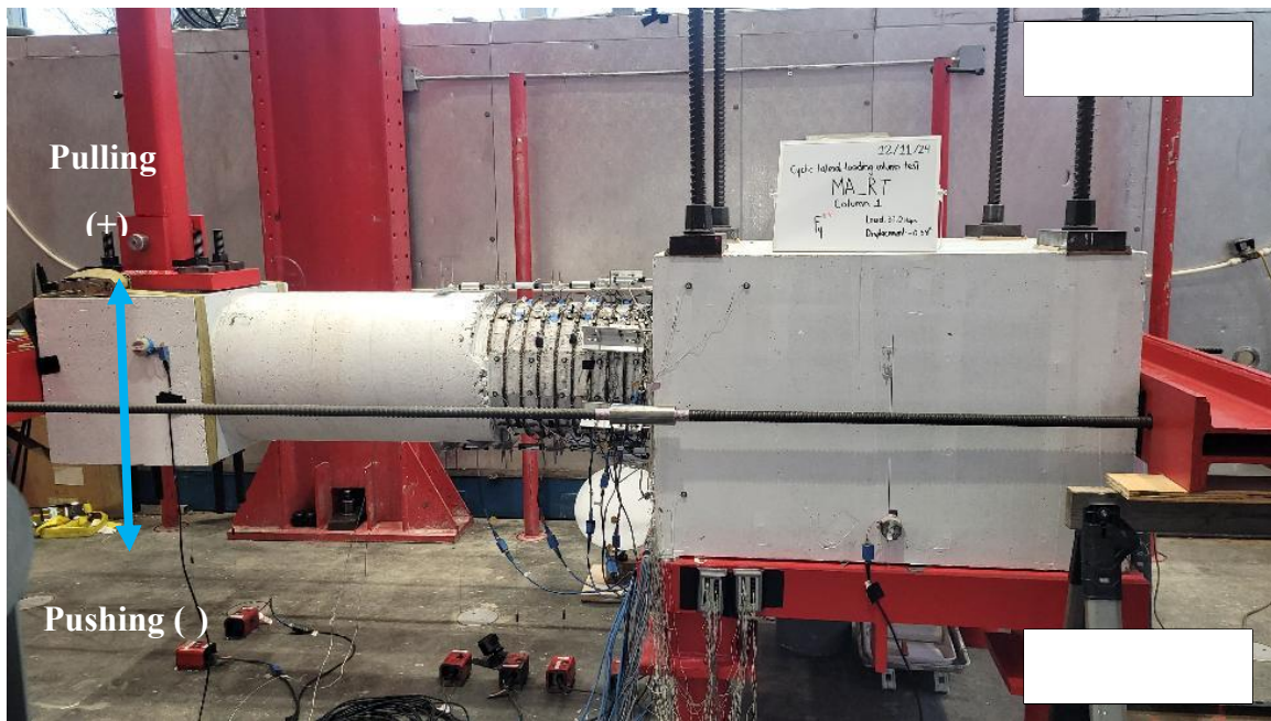
Figure 5-24 The first cycle of first yielding (pulling).
