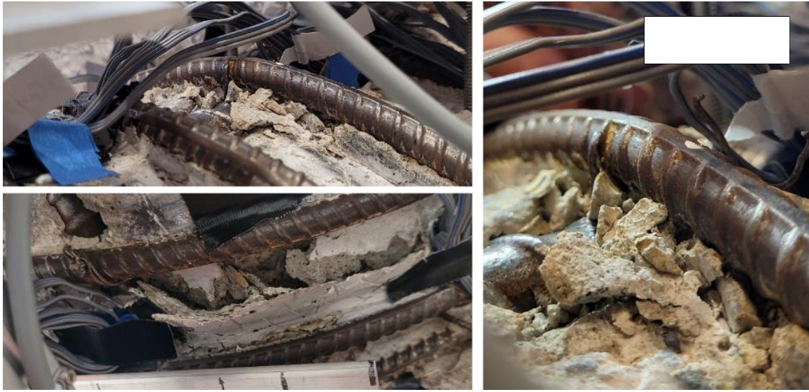
Figure 5-30 Third cycle of \mu_4 (pulling): Buckling of the top extreme bar 2T and concrete crushing
