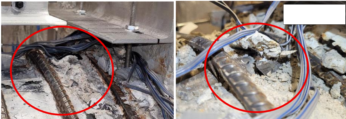
Figure 5-48 Third cycle of \mu_5 (pulling and pushing): Concrete crushing around the extreme bar 2T, followed by its fracture in the subsequent pushing cycle.
