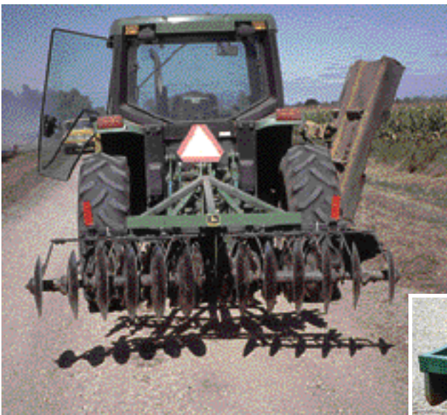
A small rear-mounted tandem disk on a mower tractor.
