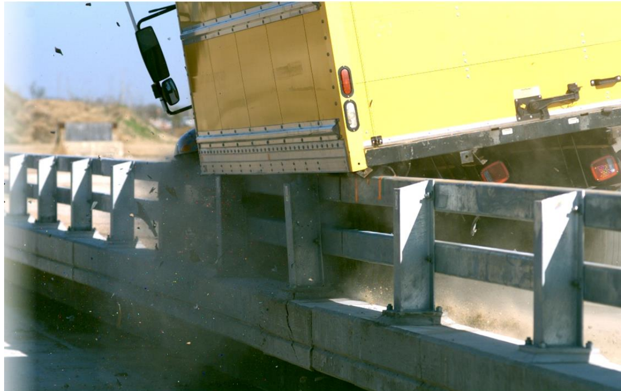
MASH Testing DOT&PF Bridge Rail Design- Texas A&M
