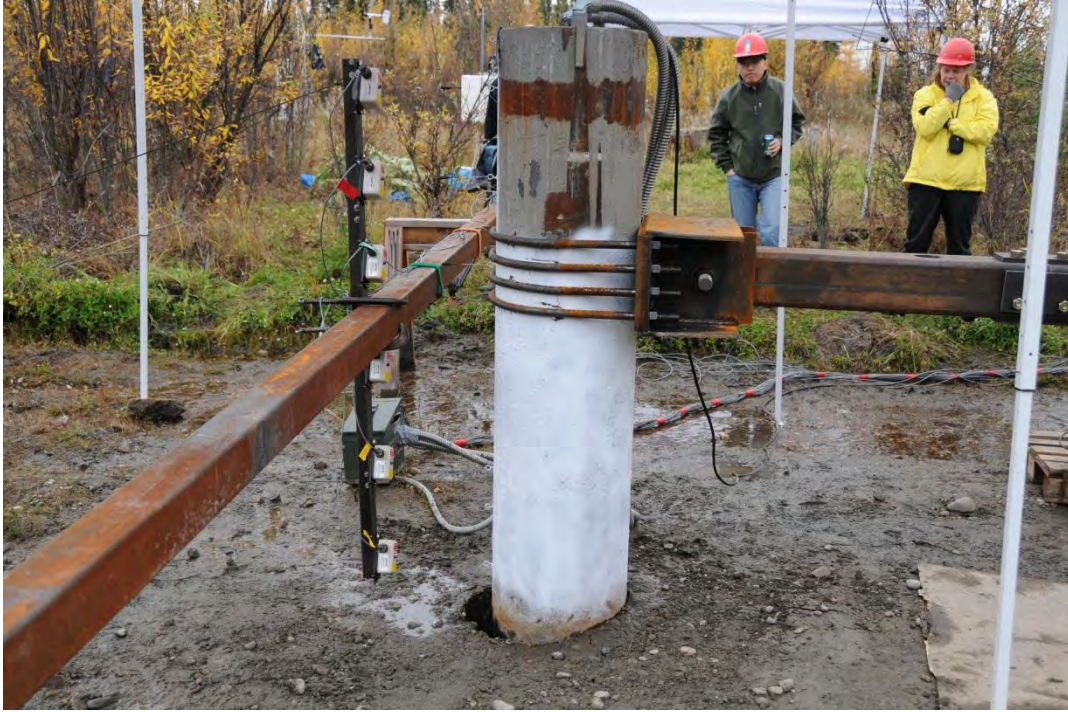
Figure 2.20: Test pile at final September load increment.
