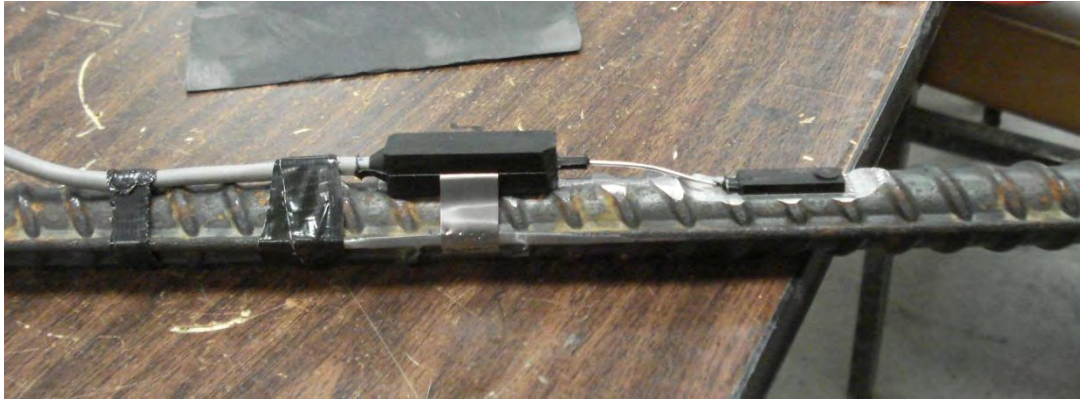
Figure 2.4: Strain gage after spot welding.
