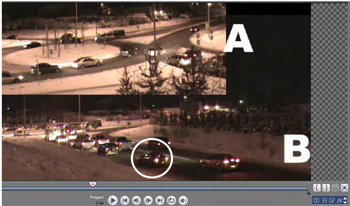
Figure 15 Picture of the arrival of the vehicle (circled) enduring the longest delay on the NB approach of the east roundabout
