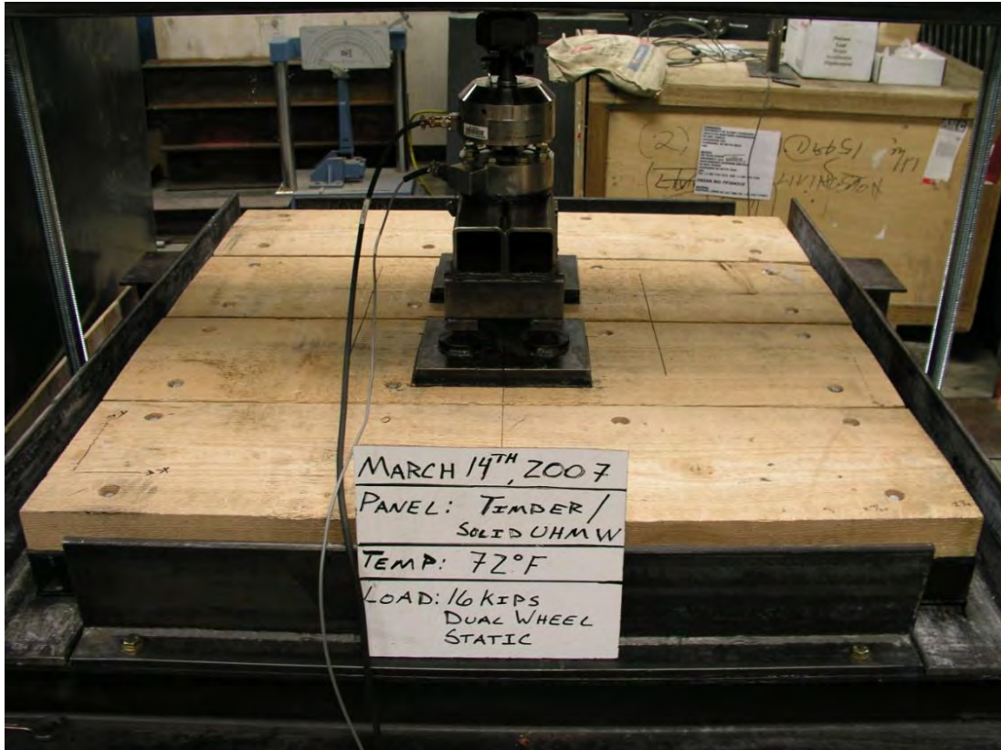
Figure 3.3 Static test for the timber on UHMW test panel.
