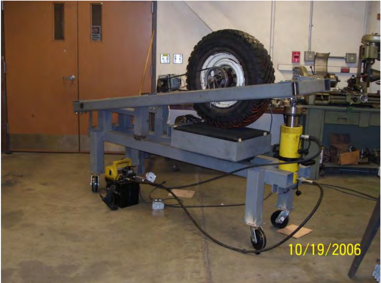
Figure 8.1 Test equipment: to measure traction and apply chain damage.
