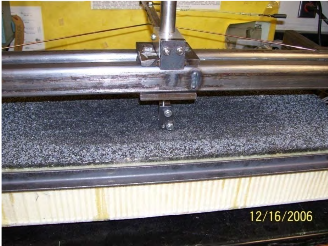
Figure 8.2 Travel arm measures x , y position; LVDT measures z position.
