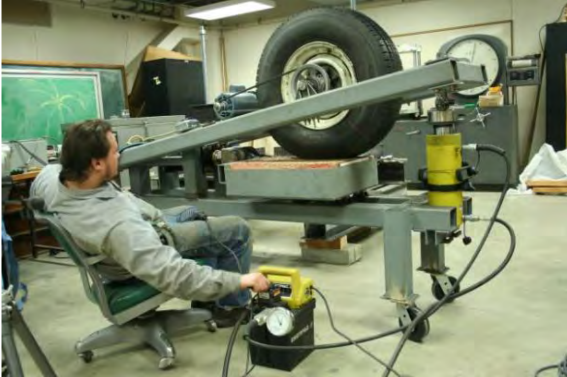
Figure 3.8 Typical traction test.
