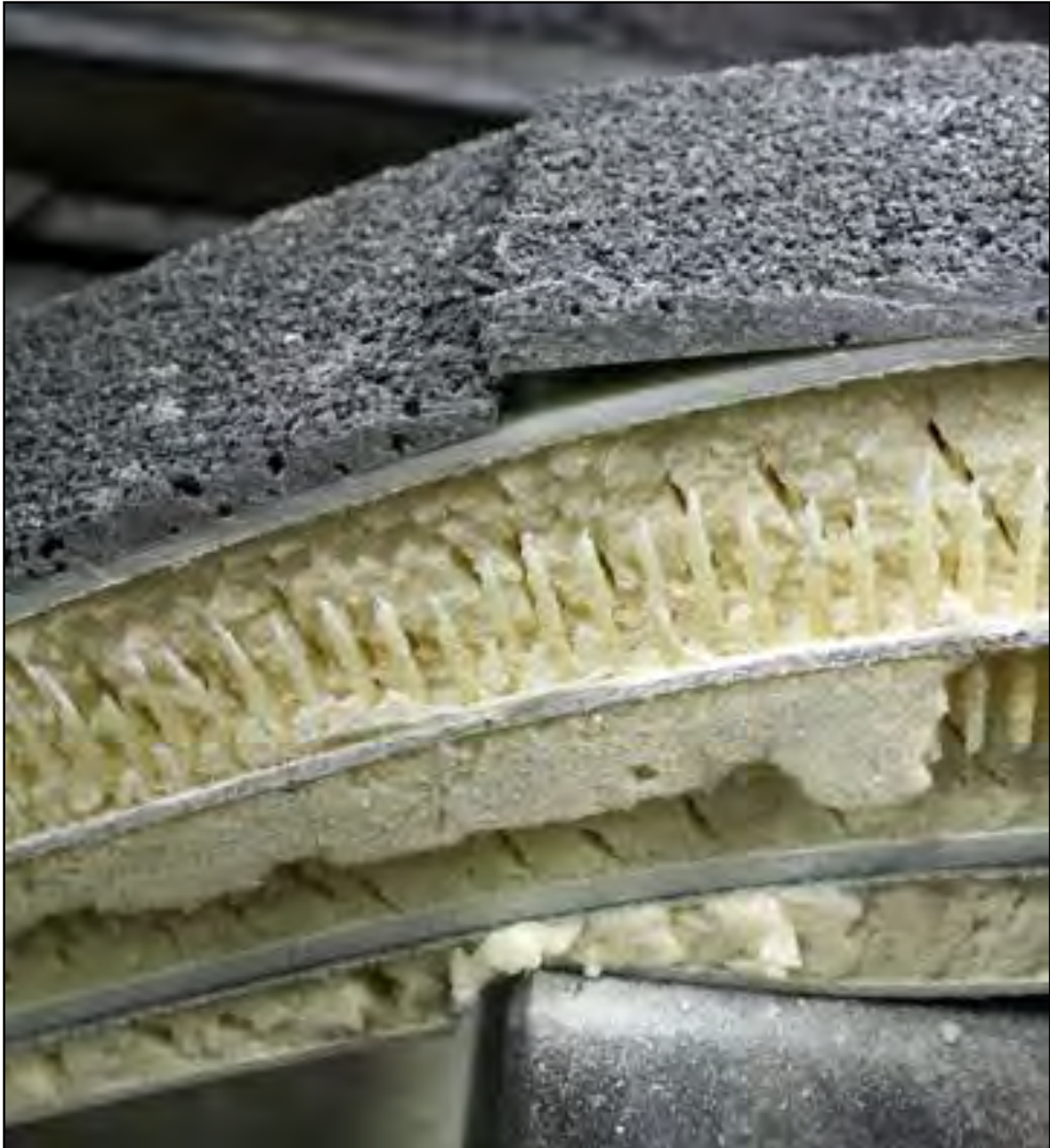
Figure 7.5 Transonite four-point bending failures.
