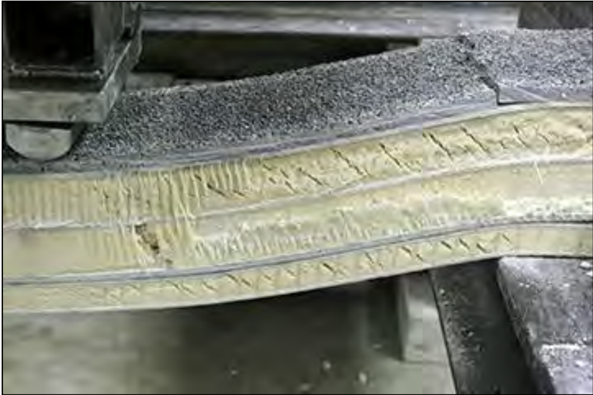
Figure 7.4 Transonite 45° shear cracks.
