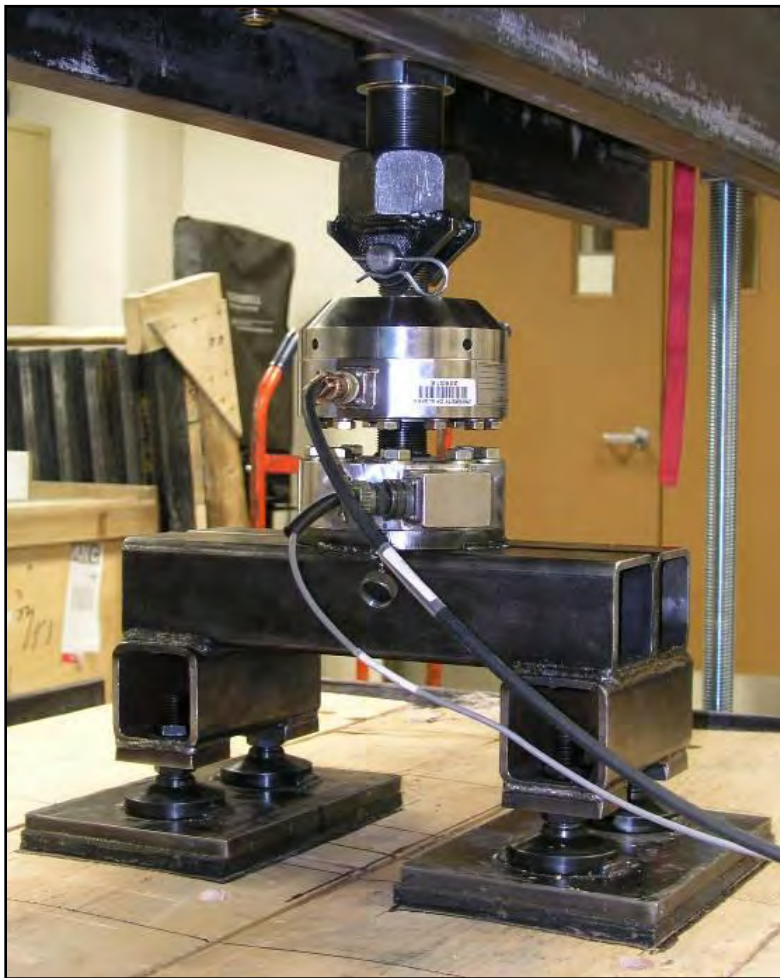
Figure A.5 Completed loading foot with load train.
