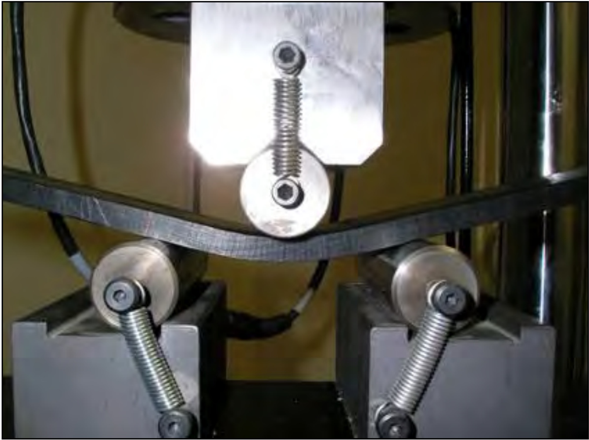
Figure 7.16 UHWM polyethylene three-point bending failure.
