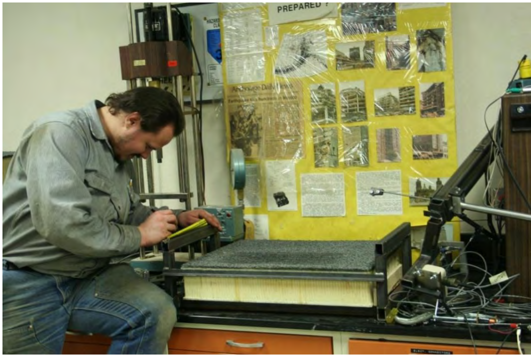
Figure 8.3 Recording surface wear for a test panel.
