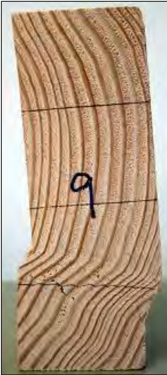
Figure 7.9 Compression perpendicular-to-grain failure.
