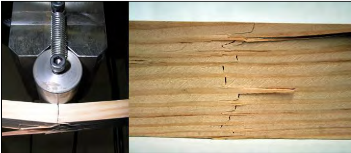
Figure 7.11 Douglas Fir three-point bending splintering tension.
