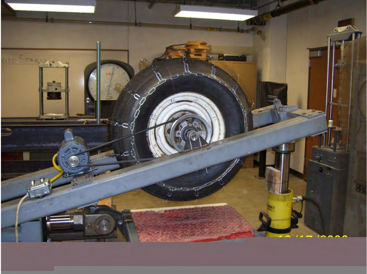
Figure 8.10 Equipment for traction, applying rolling, lashing, and drag forces.
