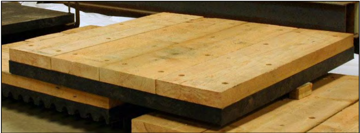
Figure A.17 Timber on solid UHMW panel.
