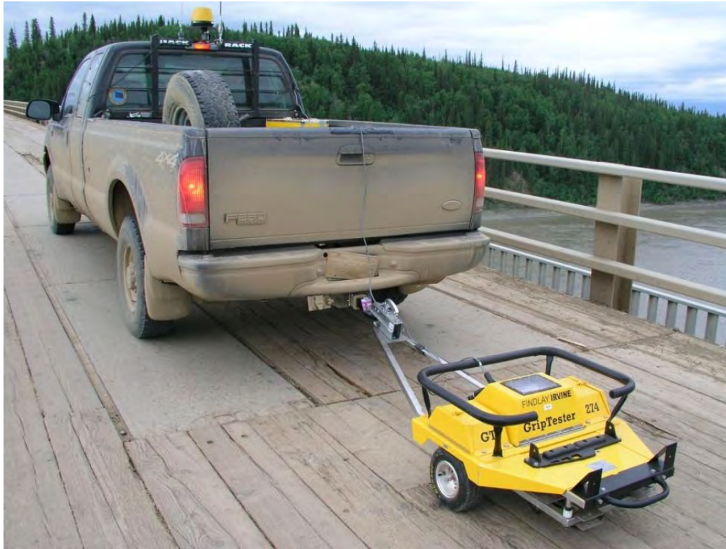
Figure 1.6 Field traction measurements using Grip Tester Type 292/16.
