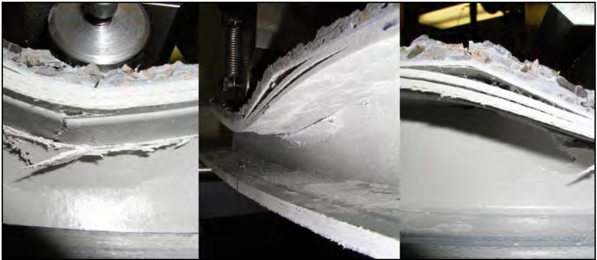
Figure 7.21 Super Panel local crushing failure in Beam 2.
