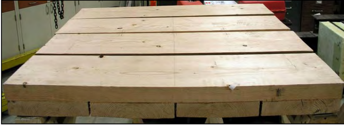
Figure 2.3 Timber on timber composite (rough sawn, two layers of 2½ in. by 12 in.
