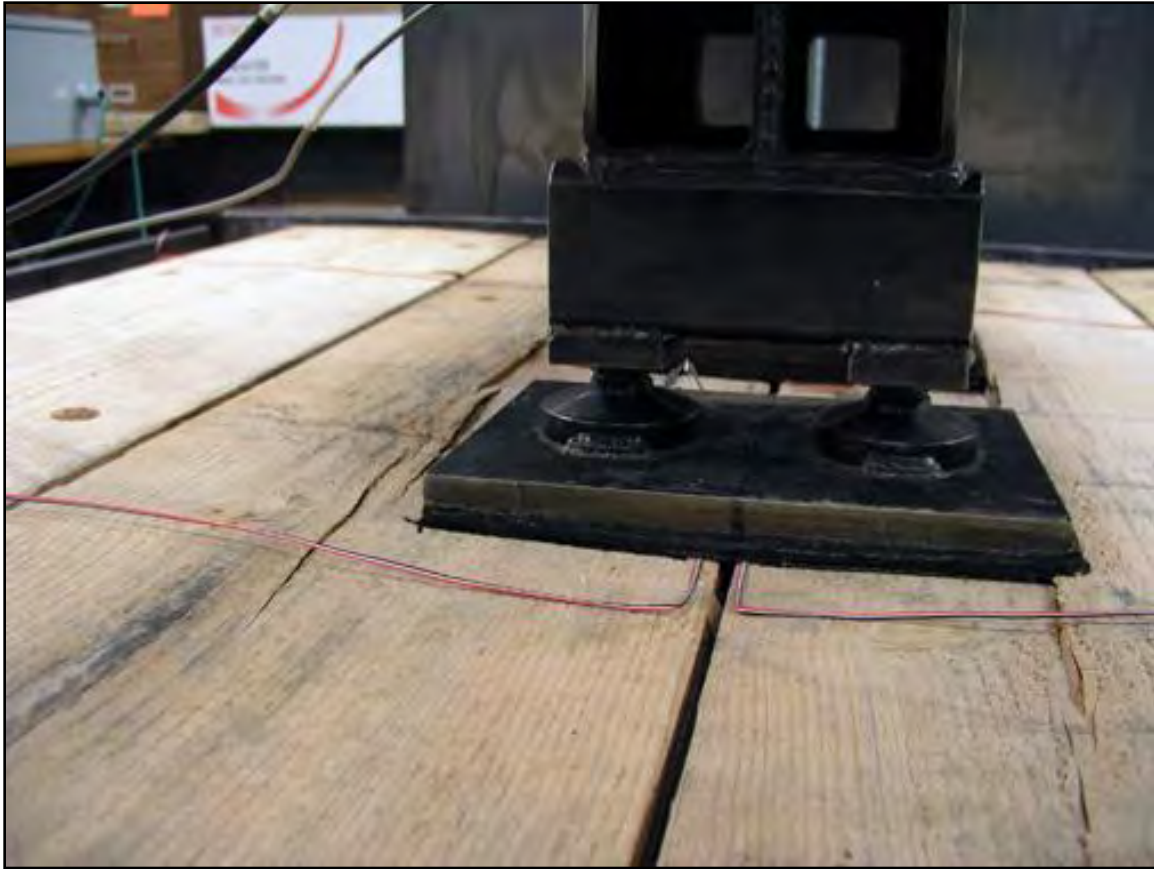
Figure 6.19 Timber on M-shaped panel with running planks cracking.
