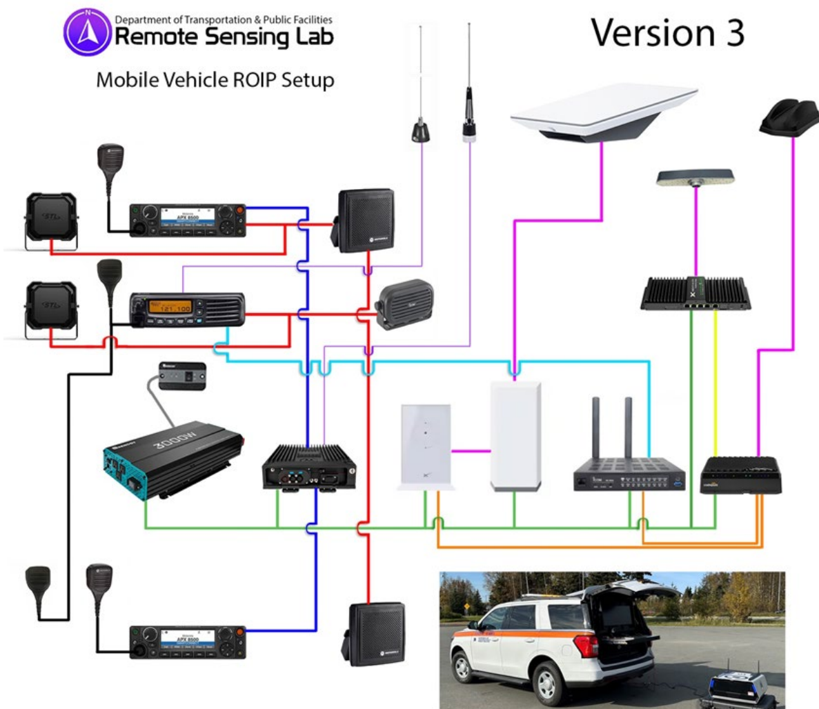
(Figure 9 – SEF Setup Diagram for Fleet Integration)
