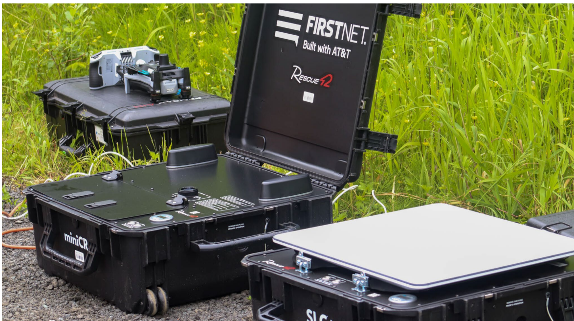
(Figure 4 - Emergency Response FirstNet Cellular Back Haul Over Starlink Enterprise)
