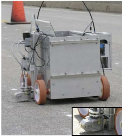
(a) Impact Echo for Delamination Detection in Concrete Decks (Gucunski & Nazarian, 2010)
