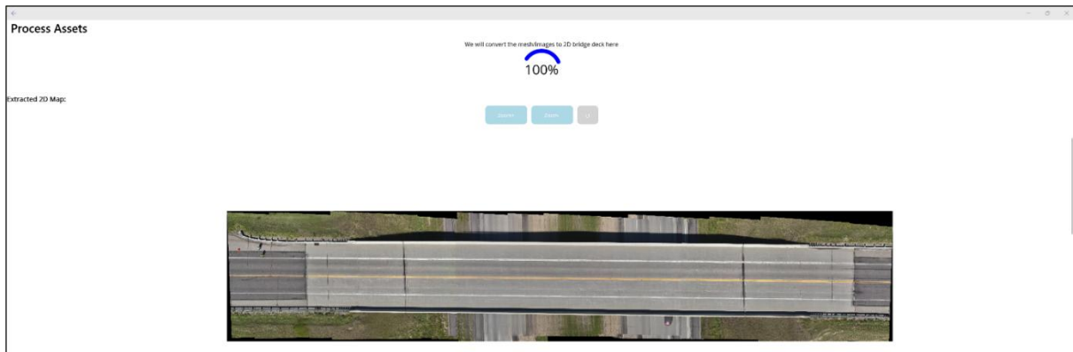
Figure 8.9 – Stitched 2D RGB Map of a Bridge Deck
