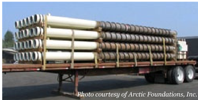
Figure 6. Thermo helix piles loaded for shipment.
