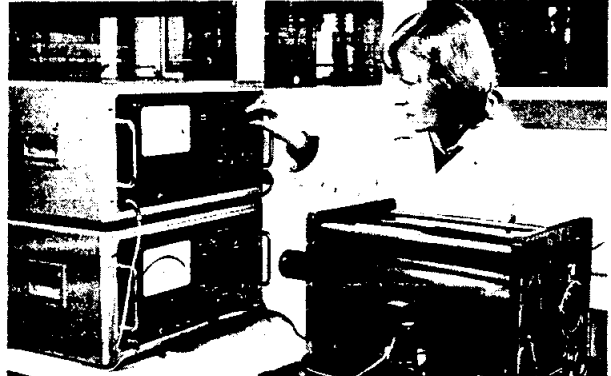
COERCIVITY MEASUREMENT. Magnetic coercivity testing of the carbide pins assures a consistent quality during pin production.
