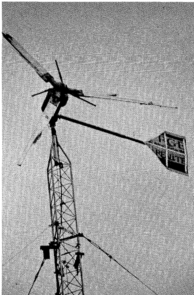
Fig. 4-10: Redwood blades (not Sitka spruce) on a foreign make machine (Source: Newell)
