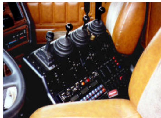
The joysticks control bed dump & hoist, plow up & down, Belly blade, and wing control.
