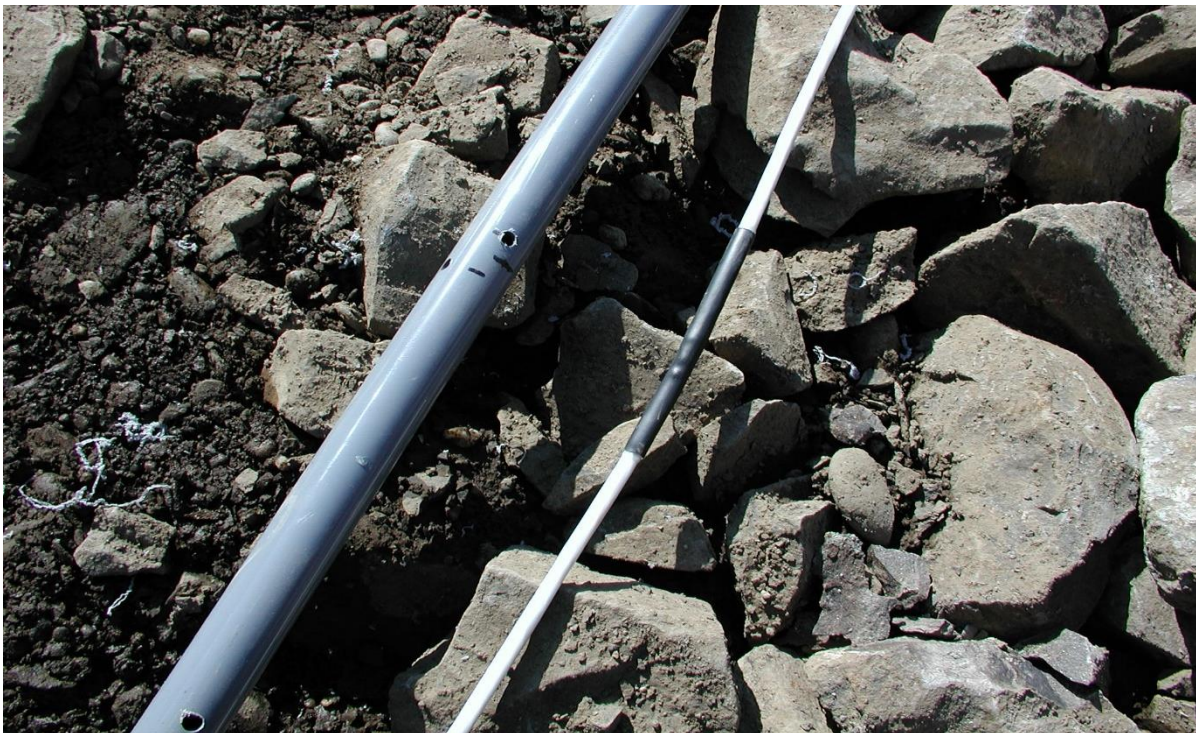
Figure 3-2 Thermistor sensor wire and vented PVC armoring tube as used in ACE areas
