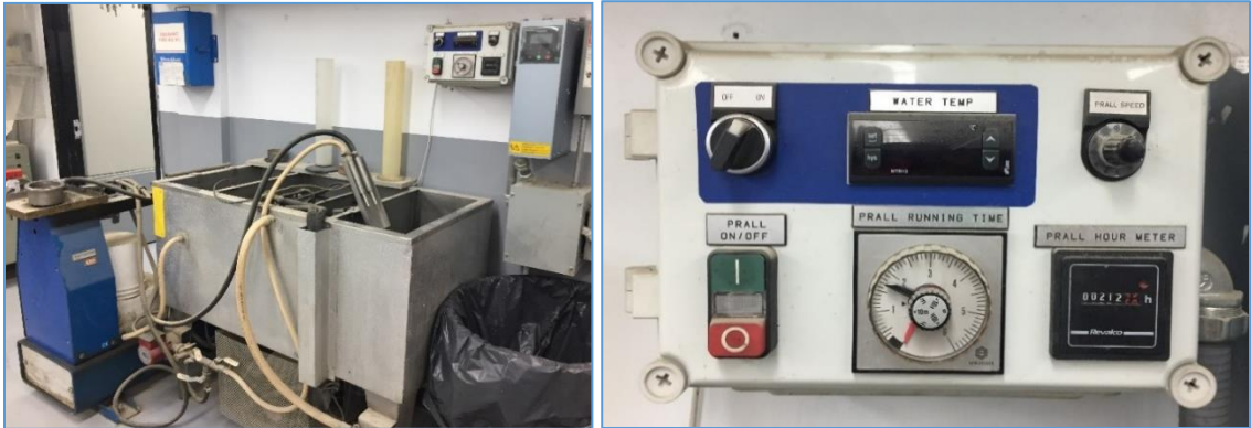
(a) Prall test setup
