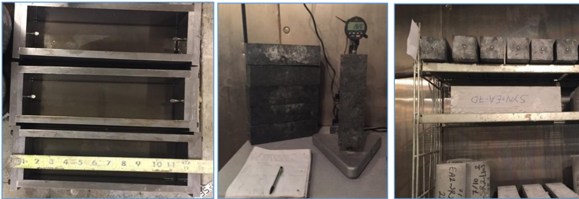
(a) Shrinkage molds (b) Measuring sample (c) Samples
