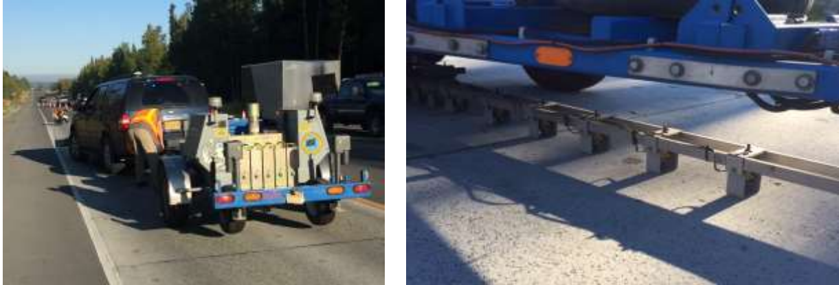
Figure 5: Falling weight deflectometer testing device used (Abaza, 2018).
