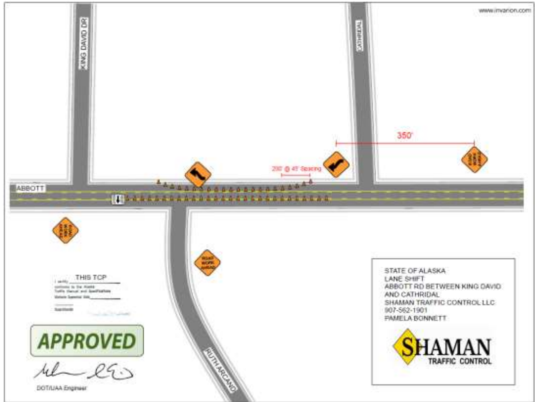
Figure 1: Traffic control plan during physical on-site testing (SHAMAN, Inc., 2018).
