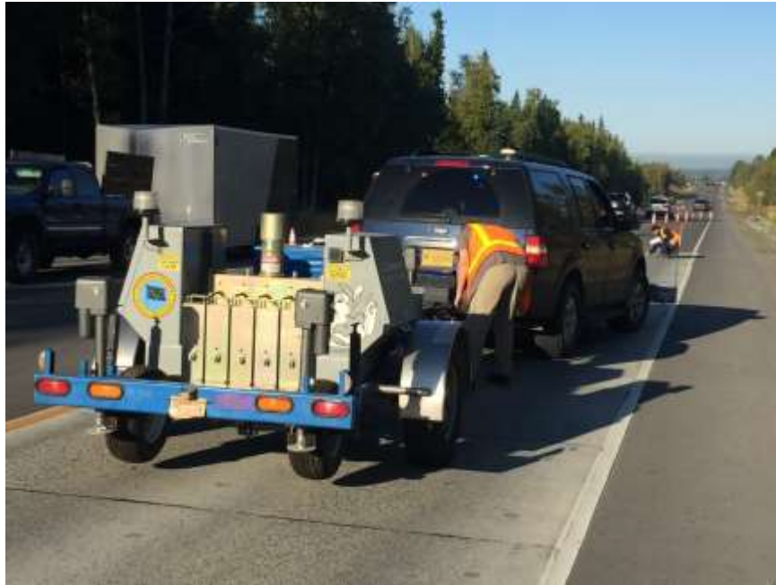
Figure A2: FWD testing on Abbott Road (Abaza, 2018)
