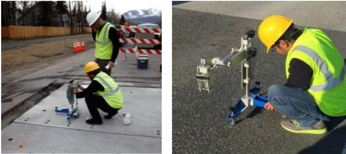
Figure 11: Skid resistance testing for SFRR and HMA (Abaza, 2017).
