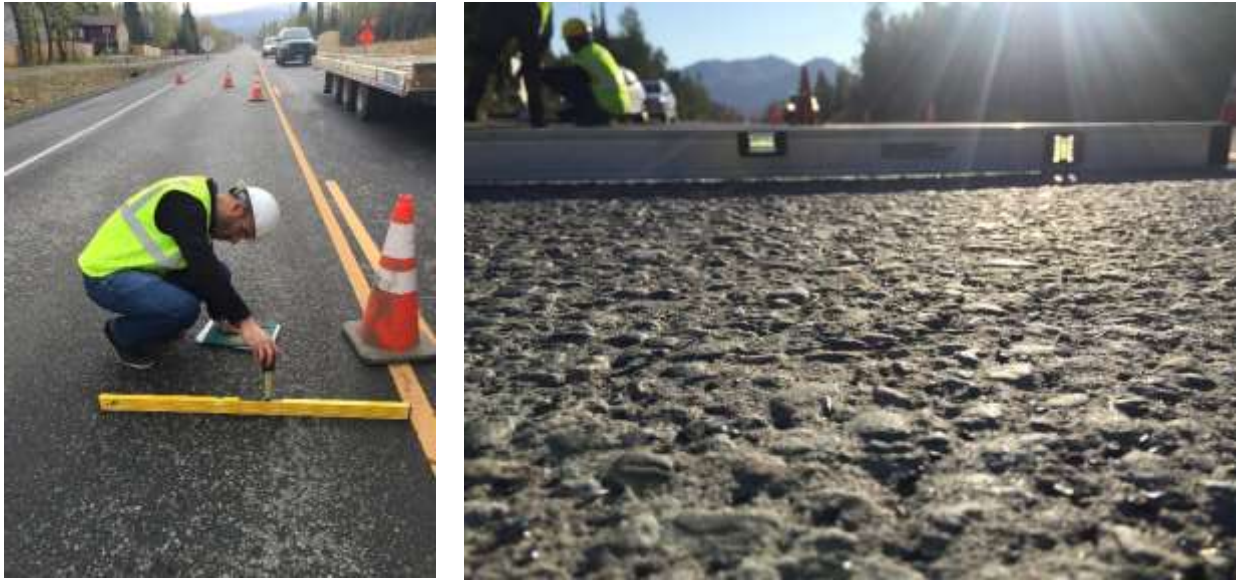
Figure 9: Rut measurements using a straight edge of adjacent HMA (Abaza, 2018).
