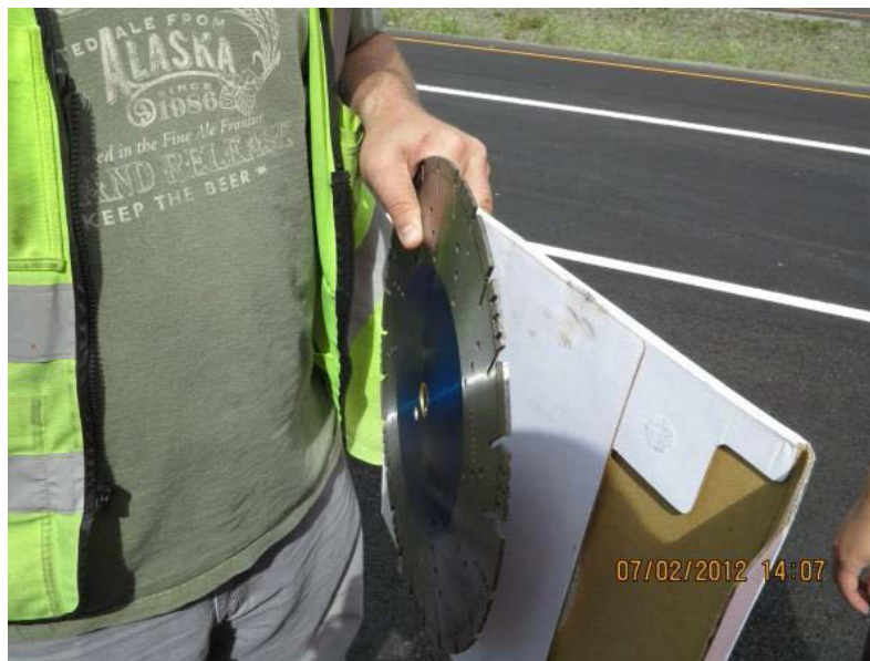
Figure 3.3 Thin diamond saw blade
