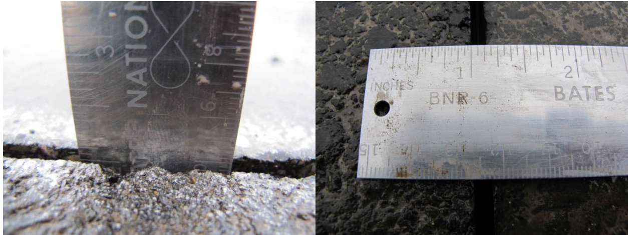
Figure 3.6 Inspection of sawn crack depth and width
