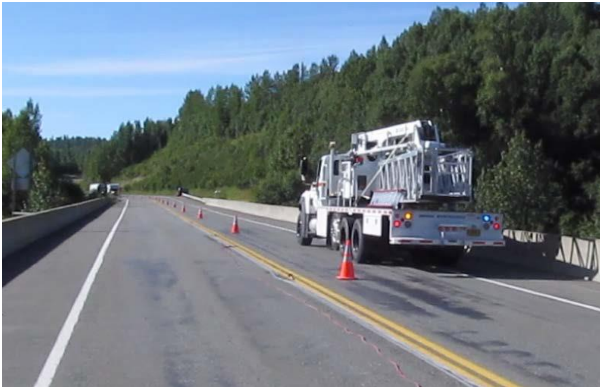
Figure I.3 A-30 boom truck traveling north for the dynamic ambient test
