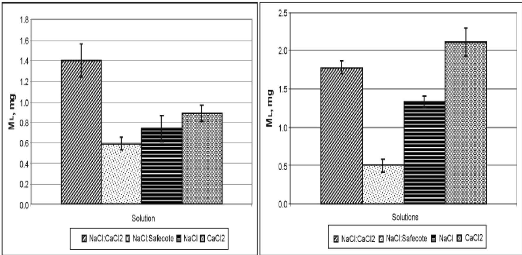
Figure A-12: Stainless steel mass loss by immersion method on left and spray on right (Petkuvienė and Paliusis 2009).
