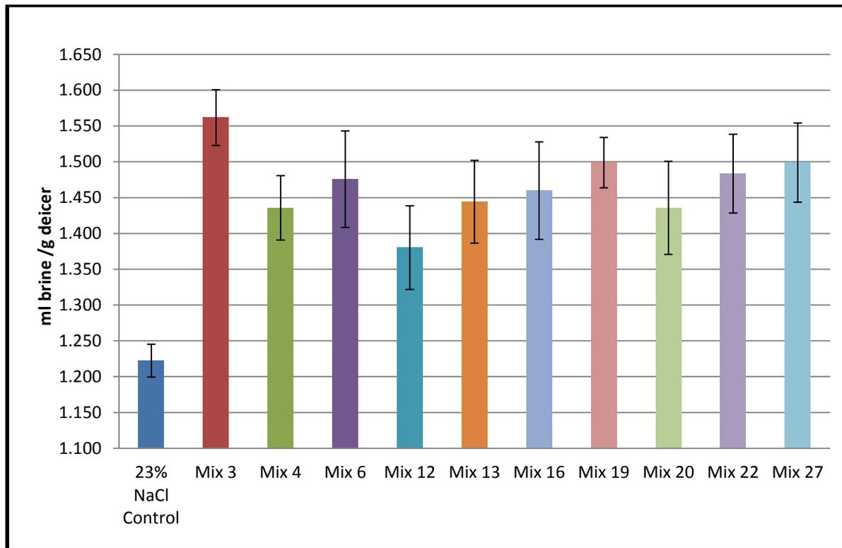
**Figure 4: Ice Melting Performance at 60 min at a temperature of 15°F.**
