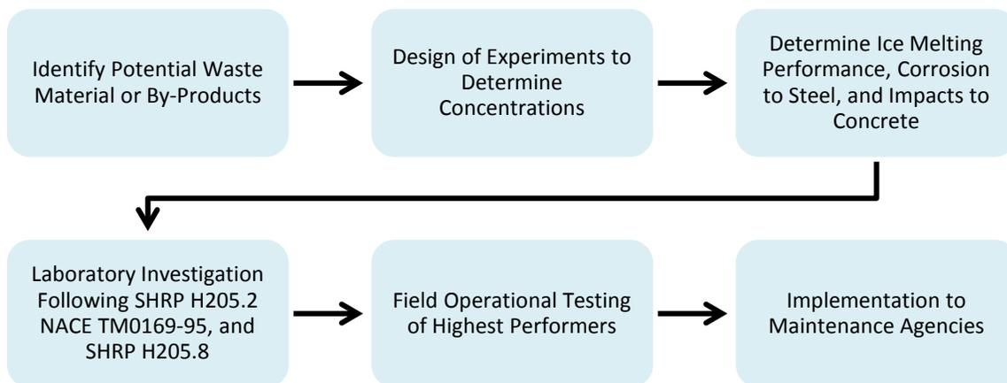
**Figure 10: Flow chart of the process of developing deicers from by-products.**
