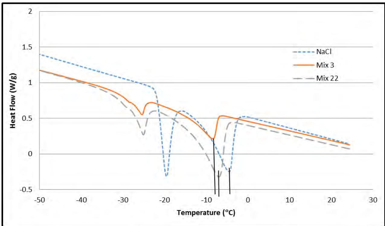
**Figure 2: DSC thermograms for 23% NaCl, Mix 3, and Mix 22.**
