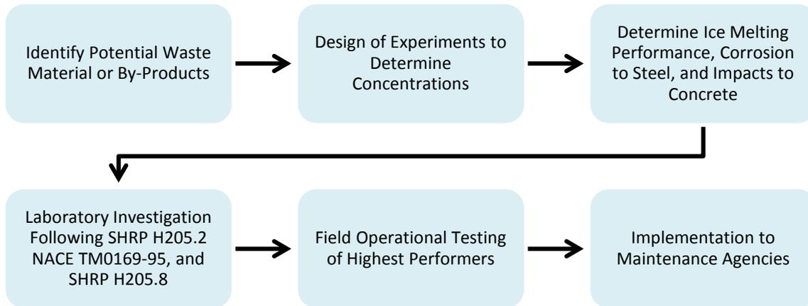
Figure 1: Process for developing alternative deicers.
