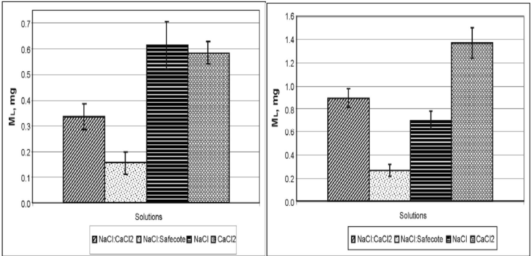
Figure A-10: Aluminum mass loss by immersion method on left and spray on right (Petkuvienė and Paliuslis 2009).
