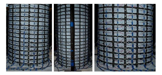
Figure 1.795 T27 – (Left) North Crack Distribution at  $(\mu_2^{+3} = 1.84")$ , (Middle and Right) Crack Distributions on the Front and Right Sides at  $(\mu_2^{-3} = -1.84")$
