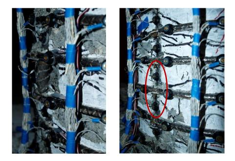
Figure 1.862 T28 – (Left) Increased Deformation in Bar N3 during ( $\mu_6^{-1} = -8.01$ "), (Right) Buckling of Adjacent Bar N2 during ( $\mu_6^{-1} = -8.01$ ")
