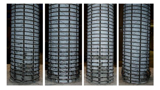
Figure 1.975 T30 – (Left to Right) North, Front, South, and Back Sides after the Test
