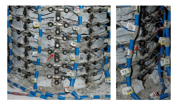
Figure 1.423 T19 – Buckling of the South Bar S3 after Reversal from  $(\mu_5^{-2})$
