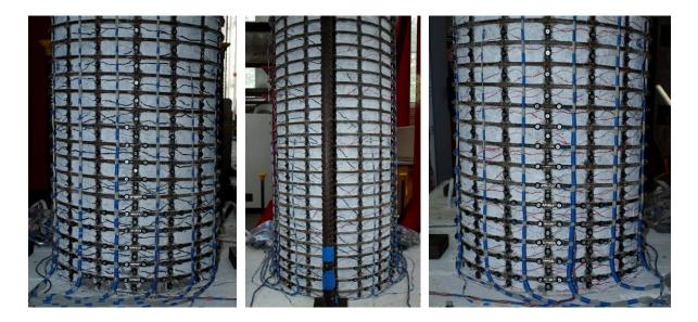
Figure 1.688 T25 – (Left) North Crack Distribution at  $(\mu_2^{+3} = 2.04")$ , (Middle and Right) Crack Distributions on the Front and Right Sides at  $(\mu_2^{-3} = -2.04")$
