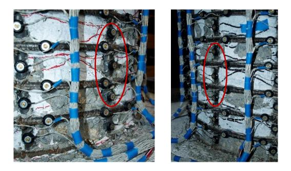
Figure 1.858 T28 – (Left) Visible Buckling of Bar S3 during ( $\mu_5^{+1} = 6.68^{"}$ ), (Right) Bar N3 Remained Visibly Straight during ( $\mu_5^{-1} = -6.68^{"}$ )
