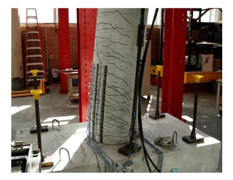
Figure 1.120 T12 – Crack Distribution at Peak Displacement ( $\mu_{10}^{3.86 \, sec} = 8.28$ ")
