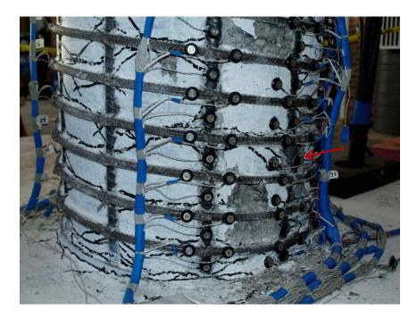
Figure 1.642 T24 – Additional Deformation in Previously Buckled Bar N3 during  $\mu_5^{-2}$
