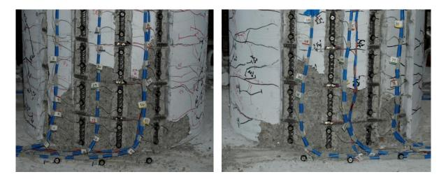
Figure 1.223 T14 – (Left) Extent of Crushing on the South Side of the Specimen during  $(\mu_4^{+3} = 3.19")$  and (Right) Extent of Crushing on the North Side during  $(\mu_4^{-3} = 3.20")$
