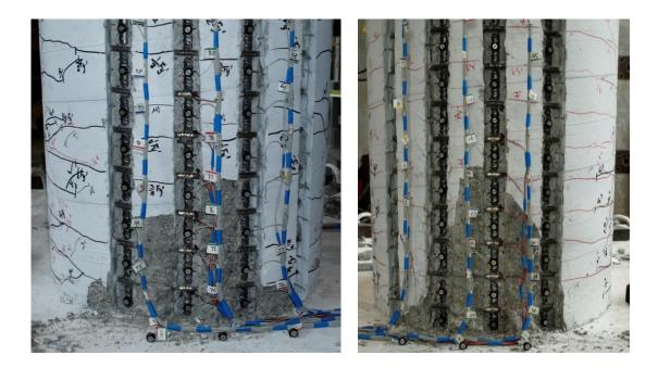
Figure 1.259 T15 – (Left) Crushing on the North Side of the Specimen during  $(\mu_3^{-3} = -2.51")$  and (Left) Crushing on the South Side during  $(\mu_3^{+3} = 2.49")$
