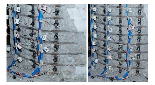
Figure 1.104 T10b – (Left) Buckling of Bar S3 after Reversal from  $(\mu_6^{-1} = -5.01")$ and (Right) Buckling of S2 after Reversal from  $(\mu_6^{-3} = -4.98")$
