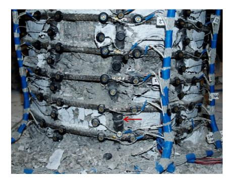
Figure 1.598 T23 – Fracture of Previously Buckled Bar N3 at 5.50" during  $\mu_7^{+2}$
