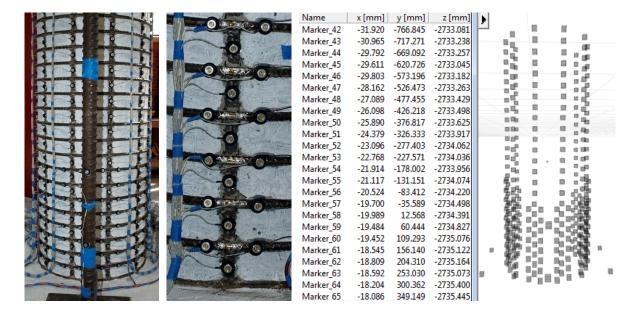
Figure 1.841 T28 – Target Marker Application and Optotrak Spatial Output
