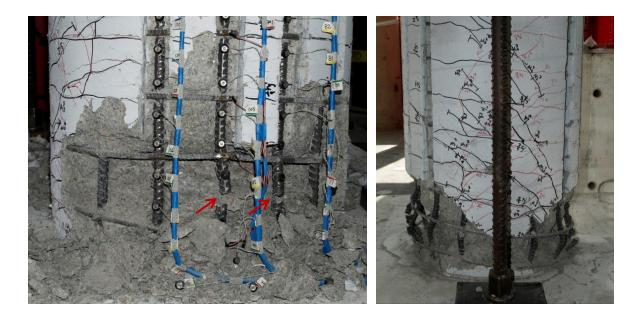
Figure 1.228 T14 – (Left) Rupture of North Buckled Bars N2 and N3 during ( $\mu_8^{+2} = 6.40^{"}$ ) and (Right) Front of the Specimen after the Conclusion of the Test
