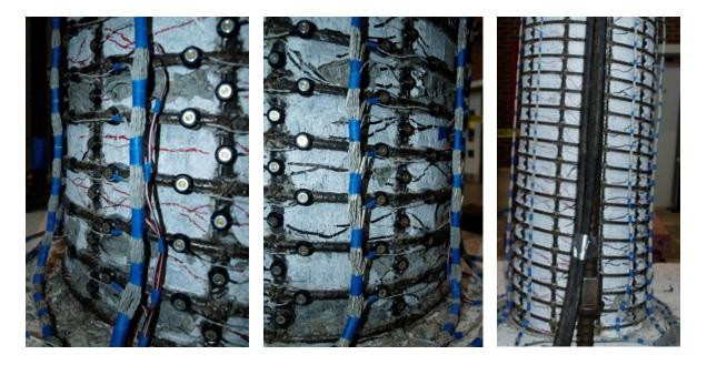
Figure 1.913 T29 – (Left) Bar S3 Remained Visibly Straight during ( $\mu_4^{+3} = 5.37^{"}$ ), (Middle) Bar N3 Remained Visibly Straight during ( $\mu_4^{-3} = -5.37^{"}$ ), (Right) Back of the Specimen at ( $\mu_4^{-3} = -5.37^{"}$ )
