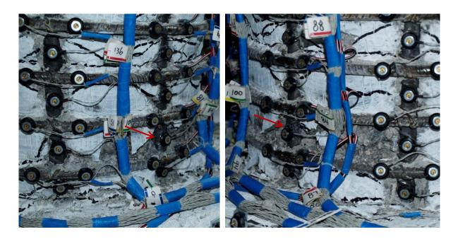
Figure 1.465 T20 – Buckling of Bar S3 after Reversal from ( $\mu_5^{-2} = -5.93''$ )
