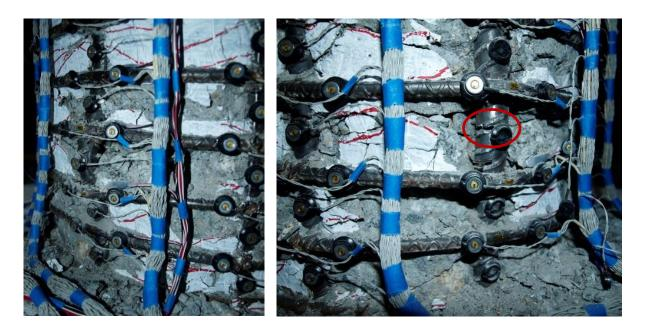
Figure 1.861 T28 – (Left) Increased Deformation in Bar S3 ( $\mu_6^{+1} = 8.00^{"}$ ), (Right) Fracture of Bar S3 during ( $\mu_6^{-1} = -8.01^{"}$ )
