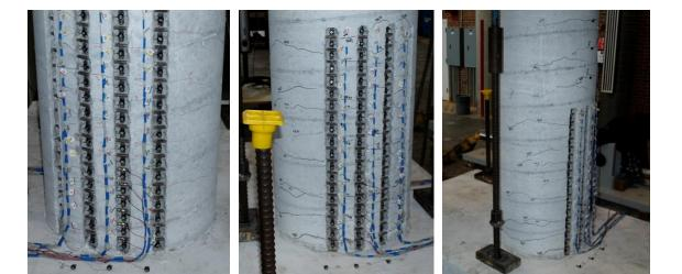
Figure 1.146 T12 – (Left) South Crack Distribution during  $(\mu_{-1.3}^{47.53 \, sec} = -1.10")$  and (Middle & Right) North Crack Distribution during  $(\mu_{2.1}^{48.83 \, sec} = 1.77")$
