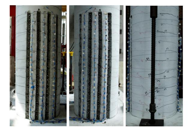
Figure 1.221 T14 – Crack Distribution after All Cycles with Actuator Load Cell Errors (No Notable Limit States Reached)
