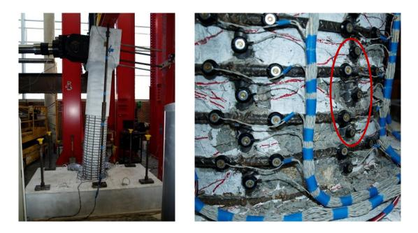
Figure 1.859 T28 – (Left) Lateral Deformation and (Right) Increased Deformation in Bar S3 during ( $\mu_5^{+2} = 6.68$ ")
