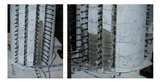
Figure 3.38 Test 6 – (Left) North Crushing observed during  $(\mu_{-2.4}^{5.08 \, sec} = -1.59")$  and (Right) Extent of South Crushing at  $(\mu_{4.6}^{10.32 \, sec} = 3.11")$
