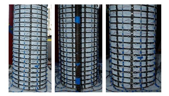
Figure 1.849 T28 – (Left) North Crack Distribution at  $(\mu_1^{+3} = 1.34")$ , (Middle and Right) Crack Distributions on the Front and Right Sides at  $(\mu_1^{-3} = -1.34")$
