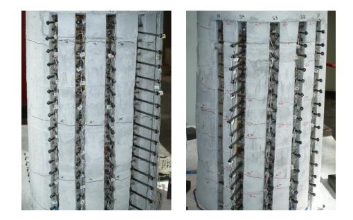
Figure 3.22 Test 4 – (Left) Crack distribution at  $(\mu_{1.0}^{1.00sec} = 0.67")$  and (Right) Crack Distribution at  $(\mu_{-1.0}^{1.32sec} = -0.66")$
