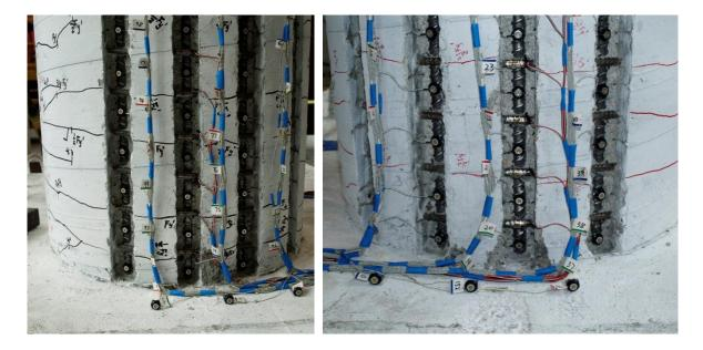
Figure 1.258 T15 – (Left) Crushing on the North Side of the Specimen during  $(\mu_{1.5}^{-3} = -1.25")$  and (Right) Crushing on the South Side during  $(\mu_2^{+1} = 1.68")$
