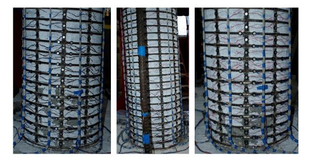
Figure 1.857 T28 – (Left) North Crack Distribution at ( $\mu_4^{+3} = 5.34^{"}$ ), (Middle and Right) Crack Distributions on the Front and Right Sides at ( $\mu_4^{-3} = -5.34^{"}$ )
