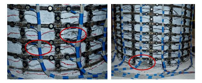
Figure 1.738 T26 – (Left) South Crushing during  $(\mu_2^{+1} = 1.99")$ , (Right) North Crushing during  $(\mu_2^{-1} = -1.99")$
