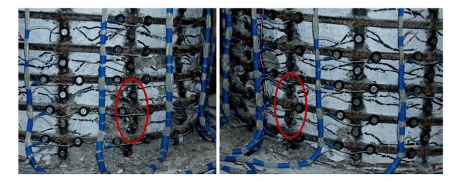
Figure 1.746 T26 – Buckling of North Bars N4 and N2 during ( $\mu_6^{-1} = -5.97$ ")
