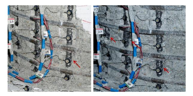
Figure 1.188 T13 – Buckling of South Reinforcing Bar S4 during  $(\mu_8^{+2} = 6.46")$  and (Right) Buckling of Bar S2 and S3 during  $(\mu_{10}^{+1} = 8.07")$
