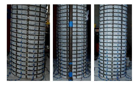
Figure 1.961 T30 – (Left) North Crack Distribution at (Fy' = 1.10"), (Middle and Right) Crack Distributions on the Front and Right Sides at (-Fy' = -1.20")
