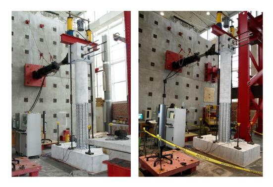
Figure 1.411 Test Setup for 11' and 13' Cantilever Length Specimens
