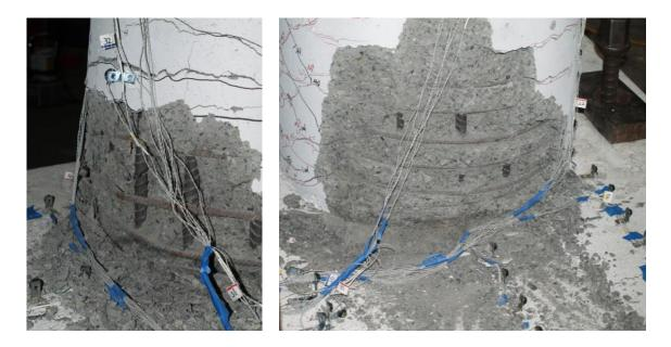
Figure 3.11 Test 2 – (Left) Fracture of Previously Buckled Bar N3 during  $(\mu_{10}^{+1} = 6.60")$  and (Right) Buckling of South Extreme Fiber Bar S3 during  $(\mu_{10}^{+2} = 6.59")$
