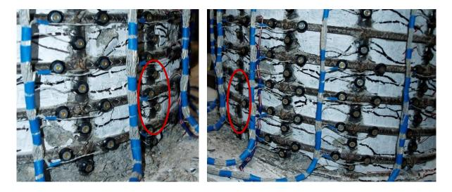
Figure 1.744 T26 – Slight Visible Buckling of Bar N3 during ( $\mu_5^{-2} = -4.99$ ")
