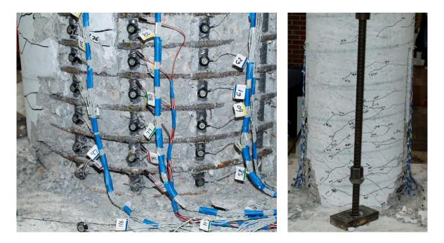
Figure 1.152 T12 – Increased Deformation in the Buckled bars toward the End of LH
