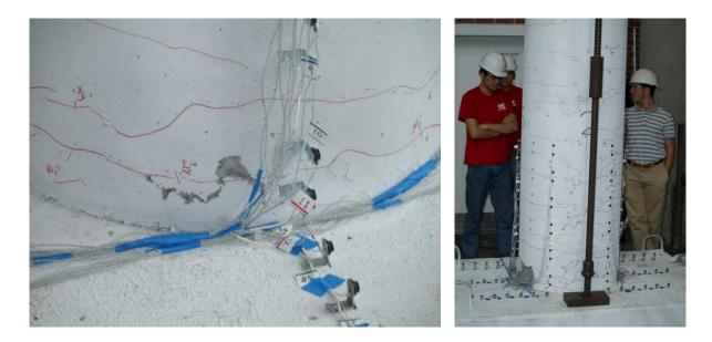
Figure 3.9 Test 2 – (Left) Initial Crushing on the South Side during  $(\mu_3^{+1} = 1.72")$  and (Right) Crack Distribution at  $(\mu_4^{-3} = -2.68")$
