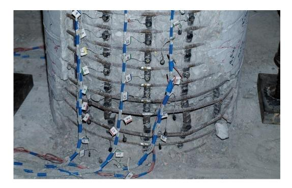
Figure 1.106 T10b – South Side after the Test (5 Buckled and 3 Ruptured Bars)
