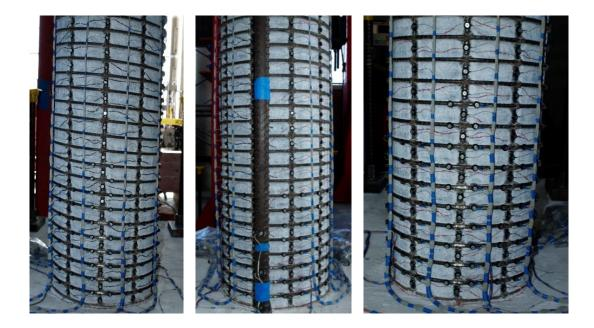
Figure 1.962 T30 – (Left) North Crack Distribution at  $(\mu_1^{+3} = 1.48")$ , (Middle and Right) Crack Distributions on the Front and Right Sides at  $(\mu_1^{-3} = -1.48")$
