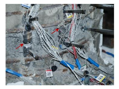
Figure 3.17 Test 3 – Fracture of Bars N2 and N3 during ( $\mu_8^{+3} = 5.37^{"}$ )
