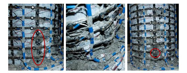
Figure 1.973 T30 – (Left) Buckling of Adjacent Bars S2 and S4 during ( $\mu_6^{+2} = 8.87$ ), (Middle) South Spiral Deformation during ( $\mu_6^{+2} = 8.87$ ), (Right) Fracture of Bar S3 during ( $\mu_6^{-2}$ )
