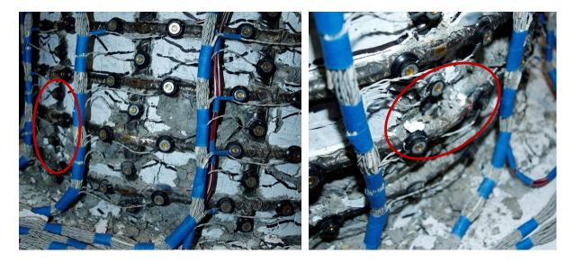
Figure 1.802 T27 – (Left) Buckling of Adjacent Bar N4 ( $\mu_5^{-2} = -4.59^{"}$ ), (Right) North Spiral Deformation at ( $\mu_5^{+3} = 4.60^{"}$ )
