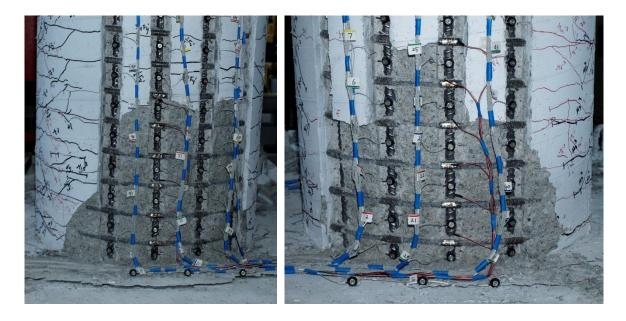
Figure 1.186 T13 – Crushing at the End of Ductility Six (Left) North and (Right) South
