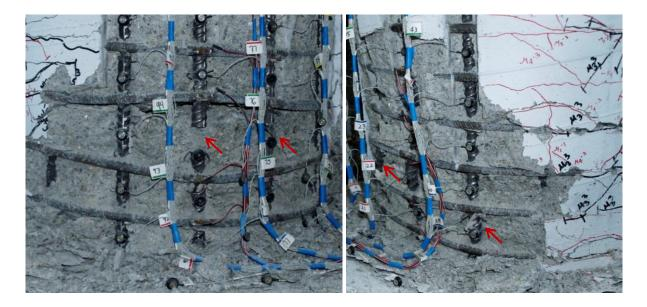
Figure 1.189 T13 – (Left) Rupture of North Reinforcement Bars N2 and N3 during  $(\mu_{10}^{+1} = 8.07")$  and (Right) Additional Deformation in South Bars during  $(\mu_{10}^{+2} = 8.06")$
