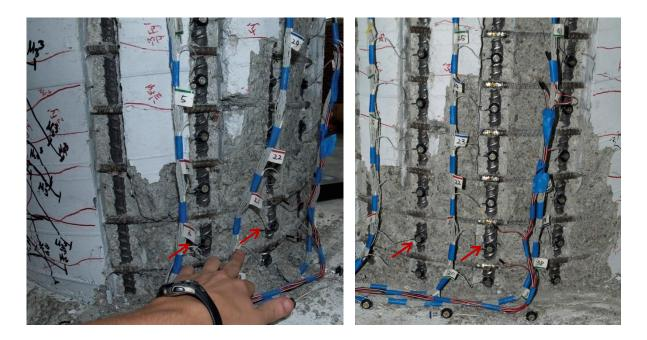
Figure 1.261 T15 – Buckling of Reinforcing Bars S2 and S3 during ( $\mu_6^{+2} = 5.00"$ )
