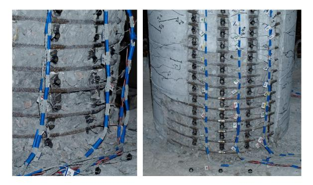
Figure 1.105 T10b – (Left) South at ( $\mu_8^{+1} = 6.64''$ ) and (Right) North Side after Test
