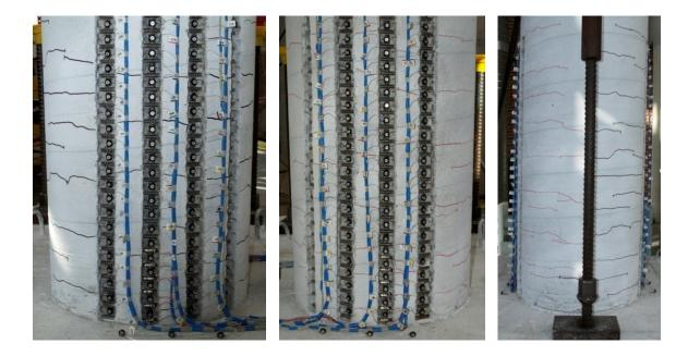
Figure 1.375 T18 – (Left) Cracks on the North Side at  $(\mu_{0.6}^{19.74 \, sec} = 0.51")$ , (Middle and Right) Crack Distribution on the South and Back Sides at  $(\mu_{-0.8}^{22.02 \, sec} = -0.66")$
