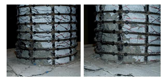
Figure 1.974 T30 – After the Test (Left) North and (Right) South Side of the Specimen
