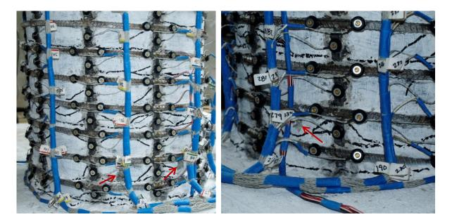
Figure 1.462 T20 – (Left) Cover Concrete Crushing on the South Side at  $\mu_3^{+1}$  and (Right) Crushing on the North Side during  $\mu_3^{-2}$
