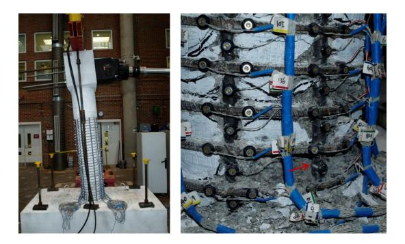
Figure 1.469 T20 – (Left) Lateral Displacement at  $(\mu_6^{+3} = 7.01")$  and (Right) Fracture of Previously Buckled Bar S3 during  $\mu_6^{-3}$
