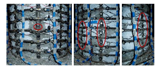
Figure 1.918 T29 – (Left) Fracture of Bar S3 during ( $\mu_6^{-1} = -8.06$ "), (Middle and Right) Buckling of Bars N2 and N3 during ( $\mu_6^{-1} = -8.06$ ")
