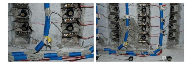
Figure 1.334 T17 – (Left) Cover Concrete Flaking Preceding Crushing on the South Side during ( $\mu_{1.6}^{12.50 \, sec} = 1.32^{"}$ ), (Right) Cover Concrete Crushing on the South Side at  $(\mu_{2.0}^{15.32 \, sec} = 1.67^{"})$
