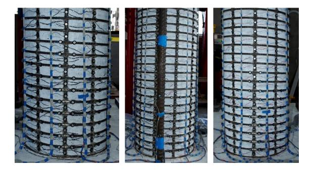
Figure 1.851 T28 – (Left) North Crack Distribution at ( $\mu_{1.5}^{+3} = 2.00^{"}$ ), (Middle and Right) Crack Distributions on the Front and Right Sides at ( $\mu_{1.5}^{-3} = -2.00^{"}$ )
