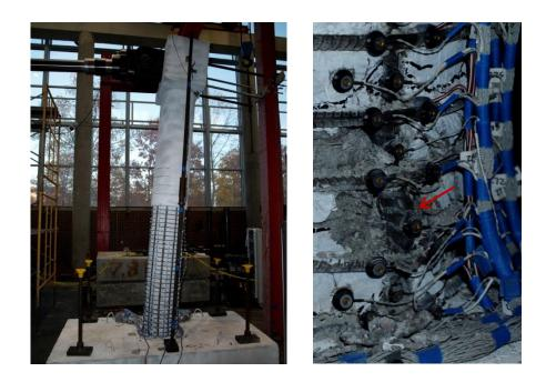
Figure 1.552 T22 – (Left) Specimen at  $(\mu_6^{+1} = 12.54")$  and (Right) Additional Deformation in Buckled Bar N3 at  $(\mu_6^{-1} = -12.53")$
