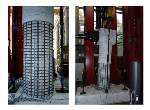
Figure 1.677 Complete Cover Concrete Blockout with Direct Application of Target Markers to Longitudinal and Transverse Steel
