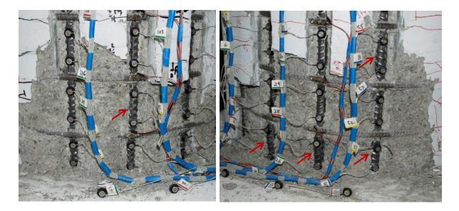
Figure 1.224 T14 – (Left) Buckling of Bar N3 during  $(\mu_6^{-1} = -4.80")$  and (Right) Buckling of South Reinforcing Bars S2, S3, and S4 during  $(\mu_6^{+2} = 4.82")$
