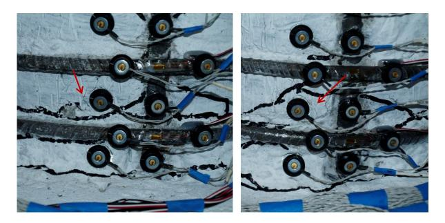
Figure 1.635 T24 – Visible Flaking of Cover Concrete which Precedes Crushing (Left) South Side during  $\mu_2^{+1}$  and (Right) North Side during  $\mu_2^{-1}$
