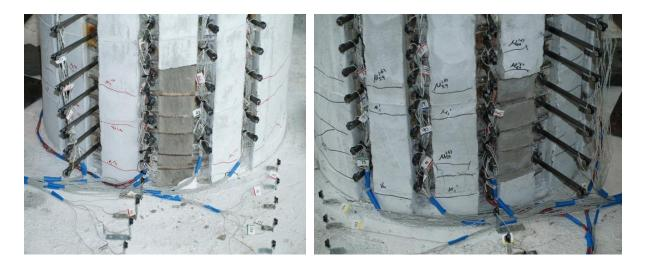
Figure 3.23 Test 4 – (Left) Crushing on the South during  $(\mu_{5.9}^{1.67sec} = 3.96")$  and (Right) Crushing on the North during  $(\mu_{-6.4}^{2.03sec} = -4.40")$
