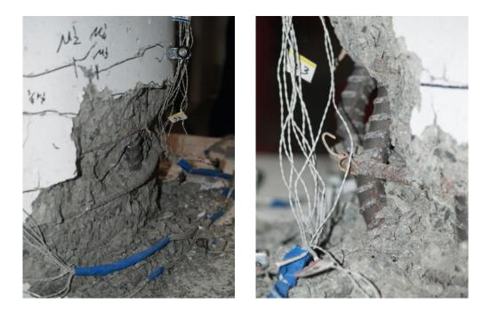
Figure 3.10 Test 2 – (Left) Buckling of Bar N3 during  $(\mu_8^{-1} = -5.39")$  and (Right) Deformation in Multiple Buckled North Bars at  $(\mu_8^{-3} = -5.36")$
