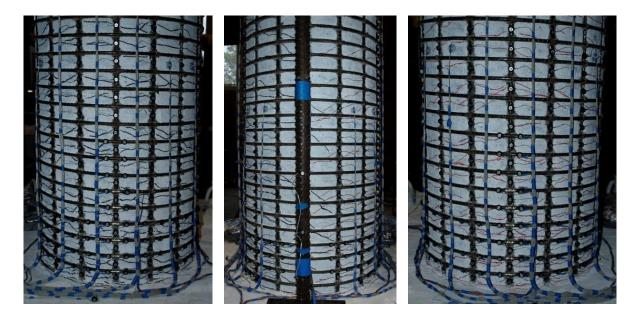
Figure 1.793 T27 – (Left) North Crack Distribution at  $(\mu_{1.5}^{+3} = 1.38")$ , (Middle and Right) Crack Distributions on the Front and Right Sides at  $(\mu_{1.5}^{-3} = -1.38")$
