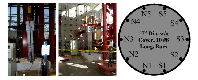
Figure 1.953 T30 – Test Setup and Cross Section Bar Designation
