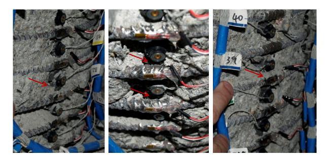
Figure 1.341 T17 – (Left) Additional Deformation in Buckled Bar N3 during ( $\mu_6^{-3} = -5.00^{"}$ ), (Middle) Spiral Deformation over North Buckled Region at ( $\mu_6^{+4} = 5.00^{"}$ ), and (Right) Additional Deformation in Buckled Bar S3 during ( $\mu_6^{+4} = 5.00^{"}$ )
