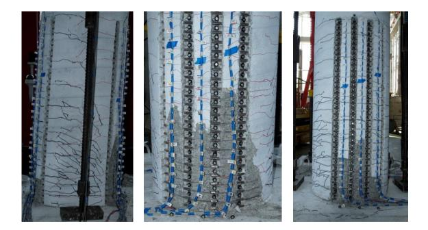
Figure 1.377 T18 – (Left) Crack Distribution on the Front Side during the Peak Cycle to  $(\mu_{9.0}^{24.40 \, sec} = 7.46")$ , (Middle) Crushing on the South Side, and (Right) Crack on the Top of the Footing on the North Side of the Column
