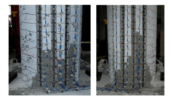
Figure 1.260 T15 – (Left) Extent of Crushing on the North Side of the Specimen during  $(\mu_6^{-1} = -5.00")$  and (Right) Crushing on the South Side during  $(\mu_6^{+1} = 5.01")$
