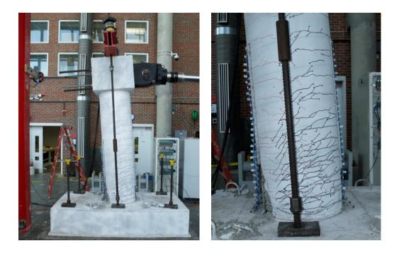
Figure 1.378 T18 – Crack Distribution at Peak Displacement ( $\mu_{9.0}^{24.40 \, sec} = 7.46$ ")
