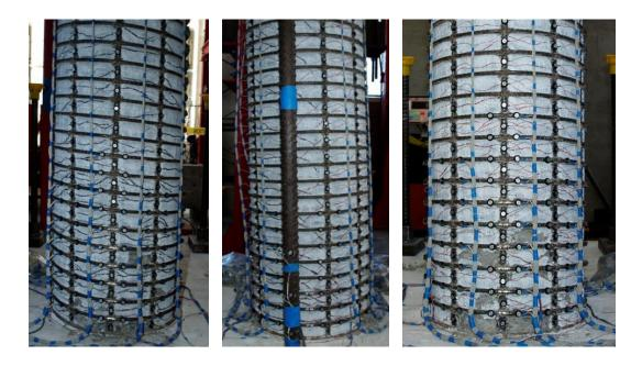
Figure 1.967 T30 – (Left) North Crack Distribution at  $(\mu_3^{+3} = 4.43")$ , (Middle and Right) Crack Distributions on the Front and Right Sides at  $(\mu_3^{-3} = -4.43")$
