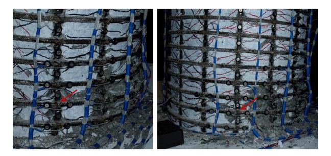
Figure 1.695 T25 – (Left) Buckling of N1 and N5 during ( $\mu_6^{-3} = -6.15$ "), (Right) Buckling of S1 during ( $\mu_7^{+1} = 7.16$ ")
