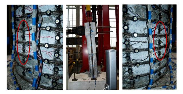
Figure 1.915 T29 – (Left) Bar S3 Remained Visibly Straight during ( $\mu_5^{+1} = 6.72^{"}$ ), (Middle) Lateral Deformation at ( $\mu_5^{-1} = -6.72^{"}$ ), (Right) Bar N3 Remained Visibly Straight during ( $\mu_5^{-1} = -6.72^{"}$ )
