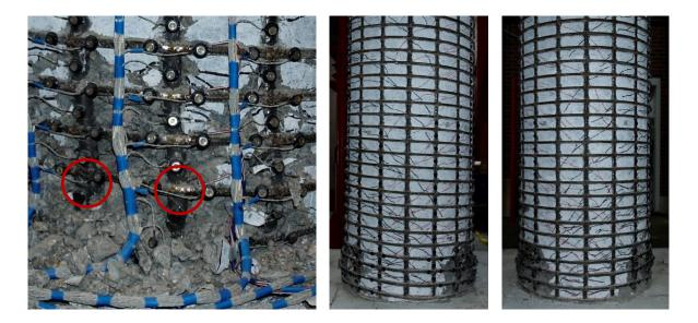
Figure 1.749 T26 – (Left) Fracture of Previously Buckled Bars N3 and N4 during  $(\mu_6^{+4} = 5.97")$ , Front (Middle) and Back (Right) After the Test
