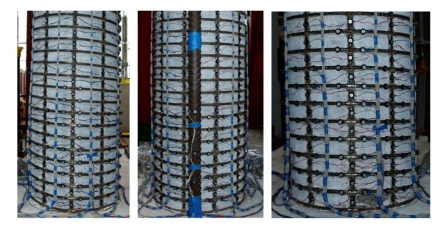
Figure 1.908 T29 – (Left) North Crack Distribution at  $(\mu_{1.5}^{+3} = 2.01")$ , (Middle and Right) Crack Distributions on the Front and Right Sides at  $(\mu_{1.5}^{-3} = -2.01")$
