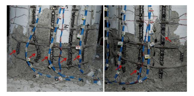
Figure 1.227 T14 – (Left) Deformation in North Buckled Bars during ( $\mu_8^{-1} = -6.39$ ") and (Right) Rupture of South Buckled Bars S2, S3, and S4 during ( $\mu_8^{-1} = -6.39$ ")
