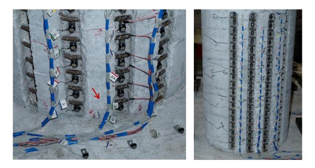
Figure 1.86 T10 – (Left) South Concrete Crushing ( $\mu_{2.0}^{13.40 \, sec} = 1.70''$ ), (Right) North
