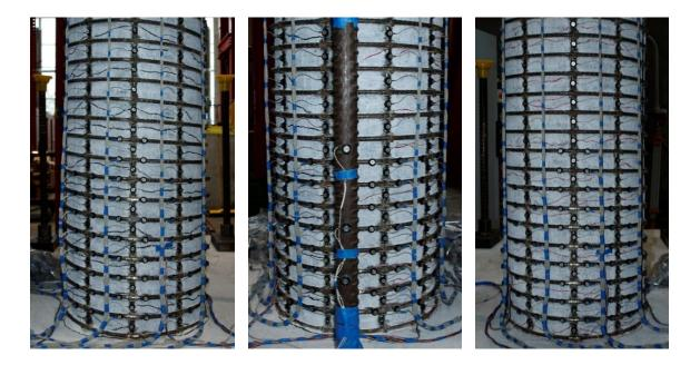
Figure 1.906 T29 – (Left) North Crack Distribution at ( $\mu_1^{+3} = 1.35$ "), (Middle and Right) Crack Distributions on the Front and Right Sides at ( $\mu_1^{-3} = -1.35$ ")
