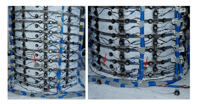
Figure 1.547 T22 – (Left) Concrete Crushing on the South Side at  $\mu_3^{+1}$  and (Right) Concrete Crushing on the North Side at  $\mu_3^{-1}$
