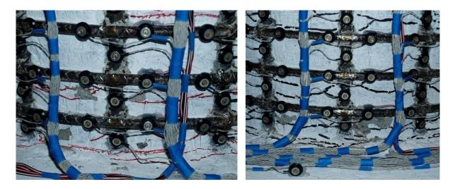
Figure 1.794 T27 – (Left) South Crushing during  $(\mu_2^{+1} = 1.84")$ , (Right) North Crushing during  $(\mu_2^{-1} = -1.83")$
