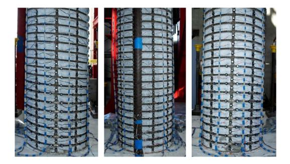
Figure 1.964 T30 – (Left) North Crack Distribution at ( $\mu_{1.5}^{+3} = 2.01$ "), (Middle and Right) Crack Distributions on the Front and Right Sides at ( $\mu_{1.5}^{-3} = -2.01$ ")
