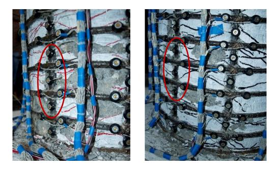
Figure 1.856 T28 – (Left) Bar S3 Remained Visibly Straight during ( $\mu_4^{+3} = 5.34^{"}$ ), (Right) Bar N3 Remained Visibly Straight during ( $\mu_4^{-3} = -5.34^{"}$ )
