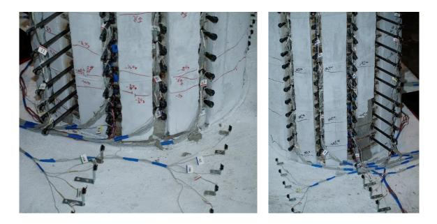
Figure 3.27 Test 5 – (Left) North Concrete Crushing at  $(\mu_{2.4}^{5.08 \ sec} = 1.59")$  and (Right) South Concrete Crushing at  $(\mu_{-2.1}^{5.4 \ sec} = -1.57")$
