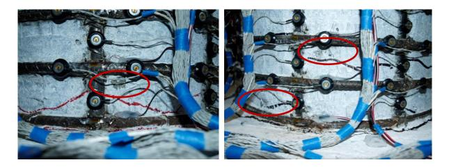
Figure 1.907 T29 – (Left) South Concrete Crushing during  $(\mu_{1.5}^{+1} = 2.01")$ , (Right) North Crushing during  $(\mu_{1.5}^{-1} = -2.02")$
