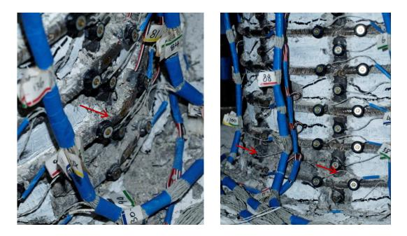
Figure 1.468 T20 – (Left) Deformation in Spiral Layers over Buckled Bar S3 during  $\mu_6^{-2}$  and (Right) Buckling of Bar S4 after Reversal from  $\mu_6^{-2}$
