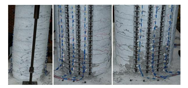
Figure 1.149 T12 – Peak Pull Cycle at  $(\mu_{-7.9}^{66.88 \ sec} = -6.53") - (Left)$  Back Side of the Specimen, (Middle) South Side, and (Right) North Side
