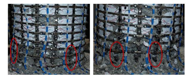
Figure 1.748 T26 – (Left) Buckling of South Bars S1 and S5 during ( $\mu_6^{+3} = 5.97^{"}$ ), (Right) Fracture of Previously Buckled South Bars S2 and S4 during ( $\mu_6^{-3} = -5.99^{"}$ )
