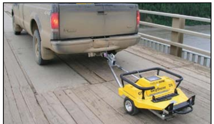
Field traction measurements using Grip Tester Type 292/16.
