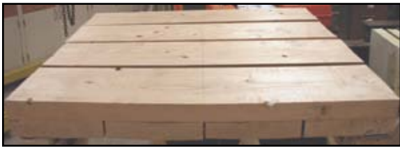
Timber on timber composite (rough sawn, two layers of 2½ in. by 12 in.).
