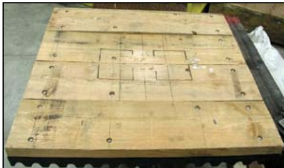
Timber driving surface lagged to UHMW M-shape.
