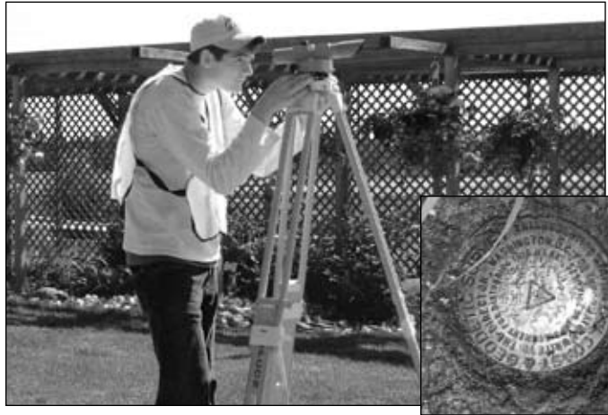
Thorton DePriest sets up his instrument (a level) as part of the survey task for the ASRA 2005 civil engineering project at the UAF Georgeson Botanical Gardens. Inset: Chena Westbase survey monument
