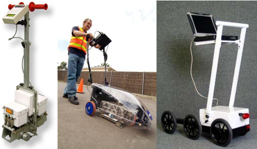
Figure 14. Examples of rolling inclinometer-based profilers (8, 9, 10)
