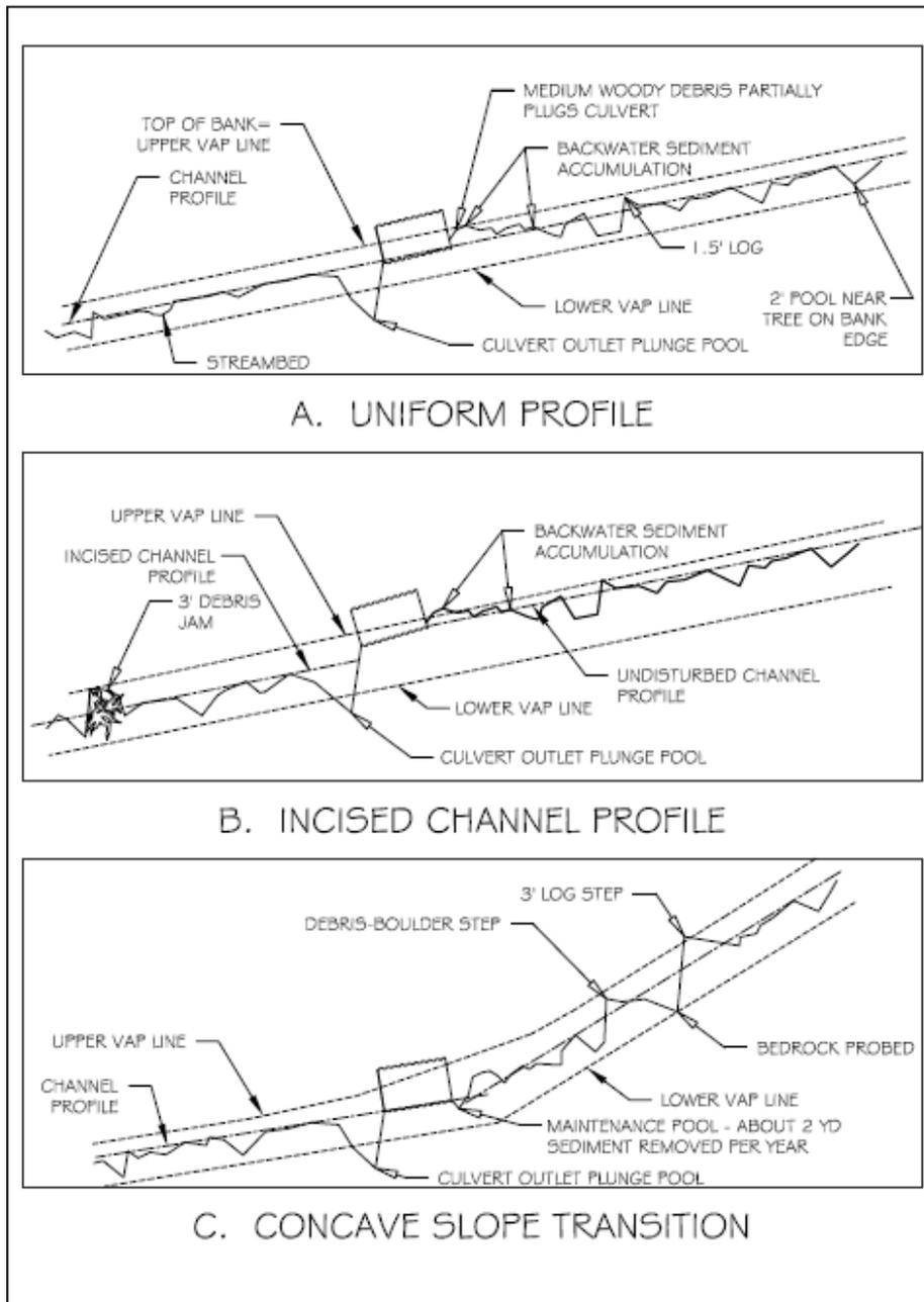
Figure 2. Vertical Adjustment Potential [USFS Stream Simulation Guide, 2008]
