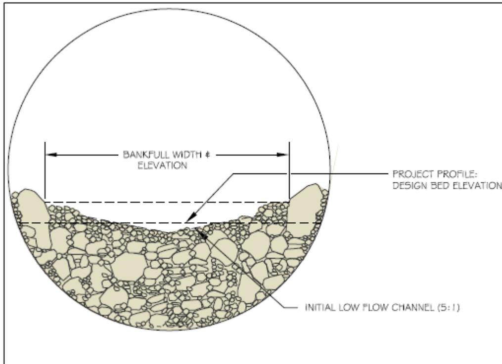
Figure 1. Low Flow Channel [[USFS Stream Simulation Guide, 2008](#)]
