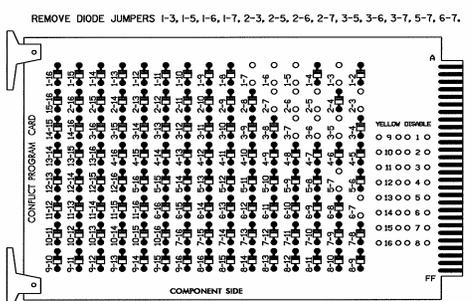
\* CARD IS PROVIDED WITH ALL DIODE JUMPERS IN PLACE. REMOVAL OF ANY JUMPER ALLOWS ITS CHANNELS TO RUN CONCURRENTLY.
