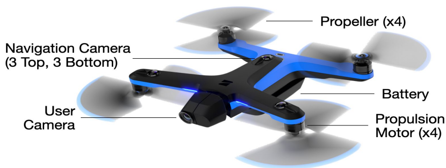
Figure 2. Location of Navigation Cameras on Skydio 2
