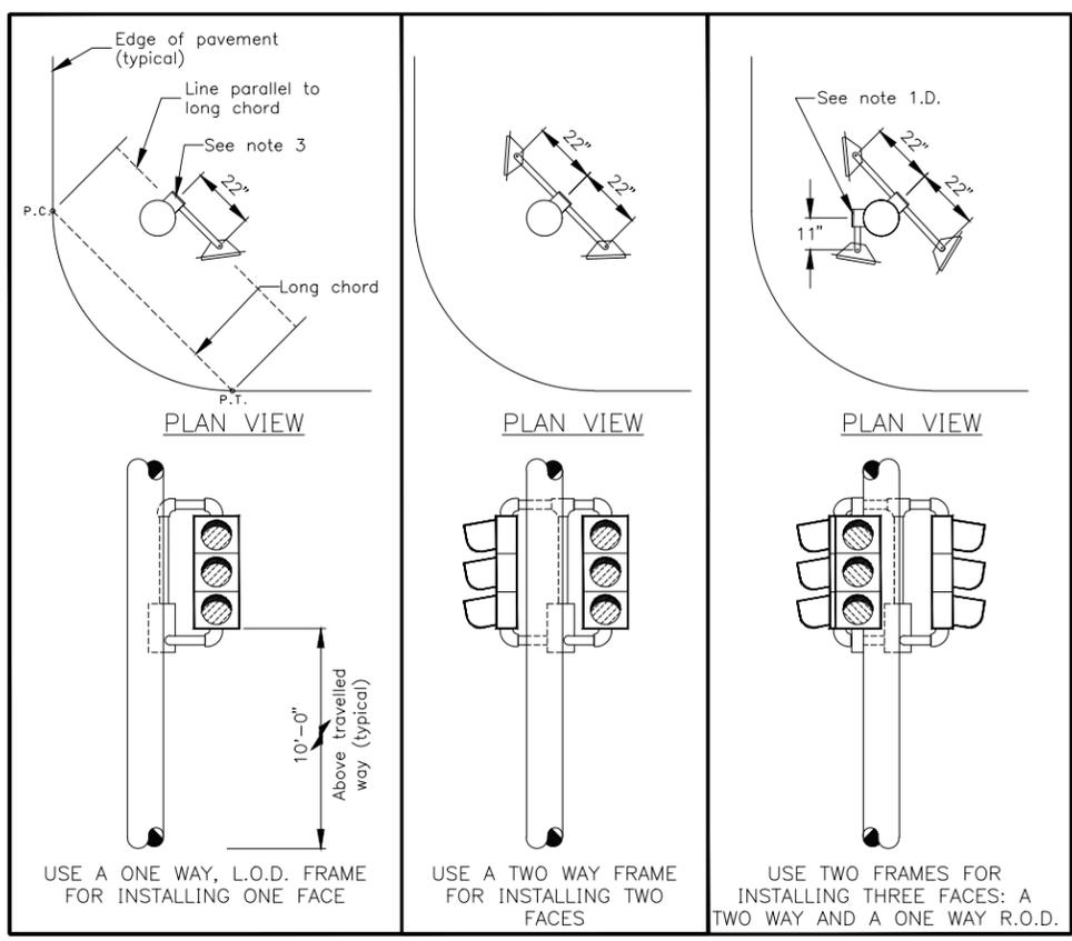
**SIDE MOUNTED SIGNAL FRAMES WITH VEHICULAR SIGNALS**
