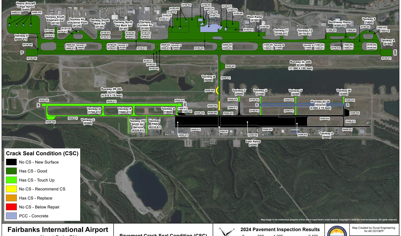
**Pavement Crack Seal Condition (CSC)**
