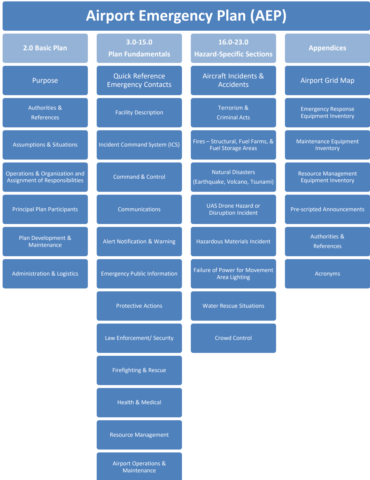
Figure 2-1: Airport Emergency Plan Structure
