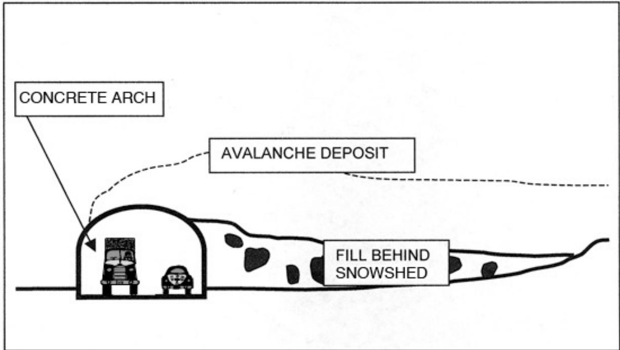
Above, a conceptual sketch of concrete arch snowshed design with backfilled ramp to reduce impact pressure on the uphill side. Depending on site configuration, backfill can also be used on the downhill side, but most snowshed designs omit the fill on that side in favor of openings or reinforced windows that provide lighting and ventilation.
