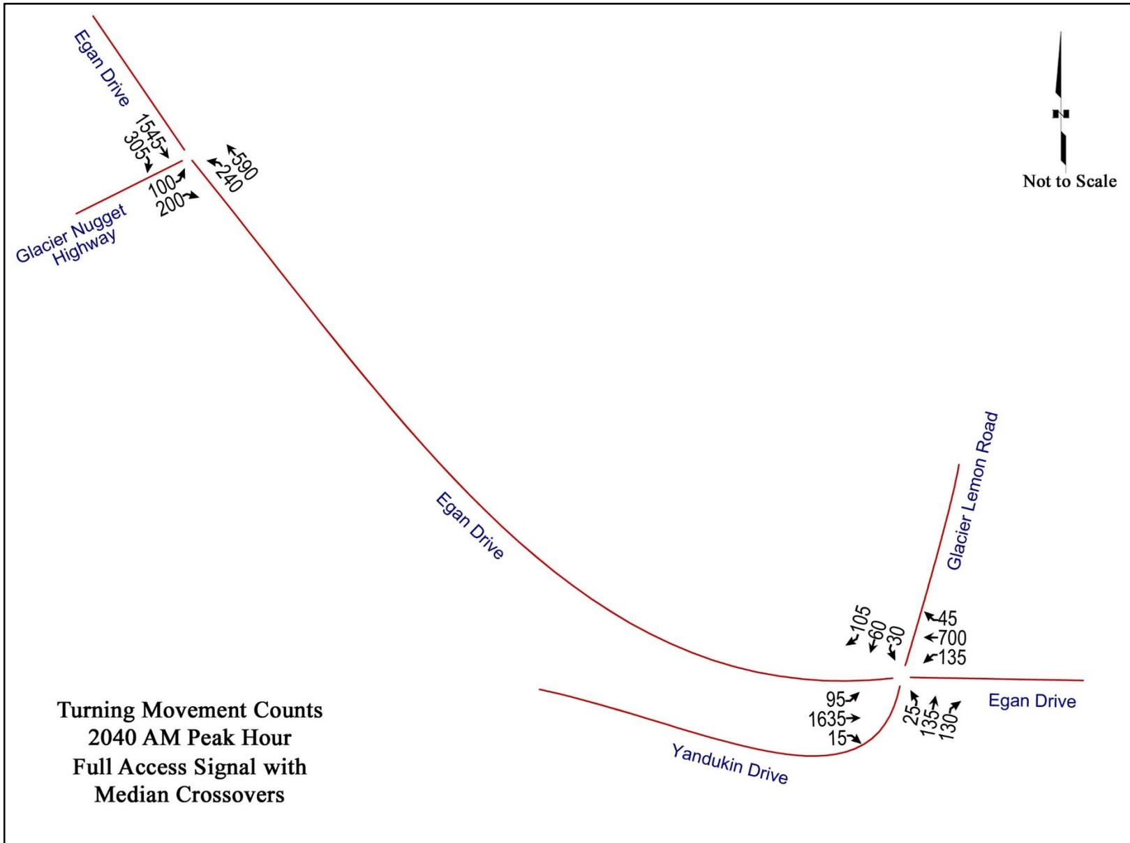
Figure D-5: Turning Movement Volumes – Full Access Signal with Median Crossovers, 2040 AM Peak
