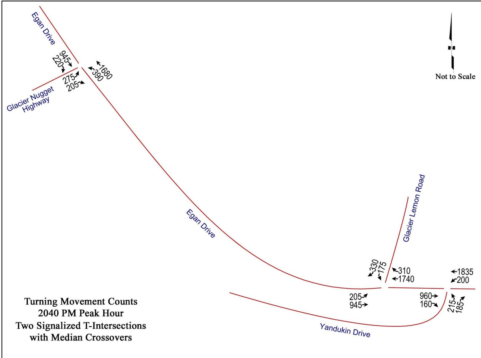
Figure D-10: Turning Movement Volumes – Two Signalized T-Intersections with Median Crossovers, 2040 PM Peak
