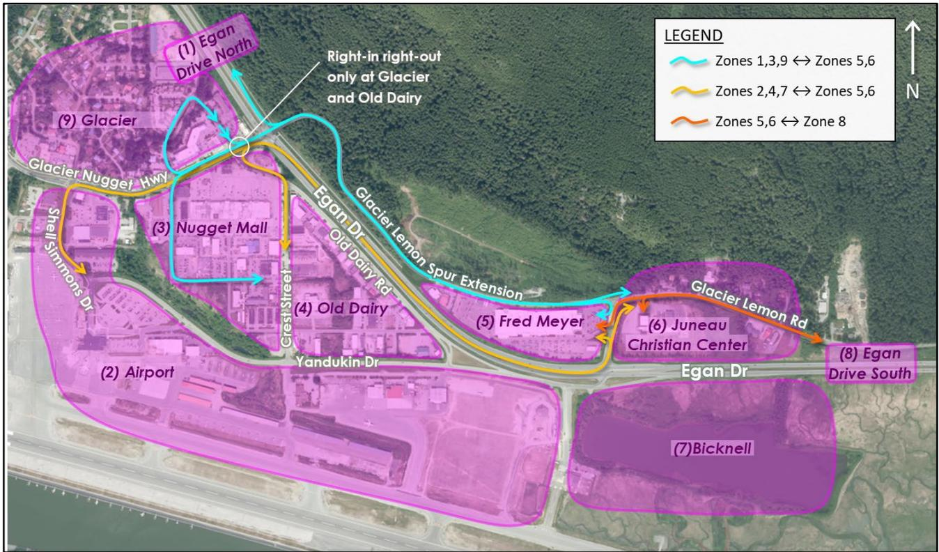
**Figure 20: Routing for No Build, Mobility, and Partial Access Signal Alternatives with Glacier Lemon Spur Extension**
