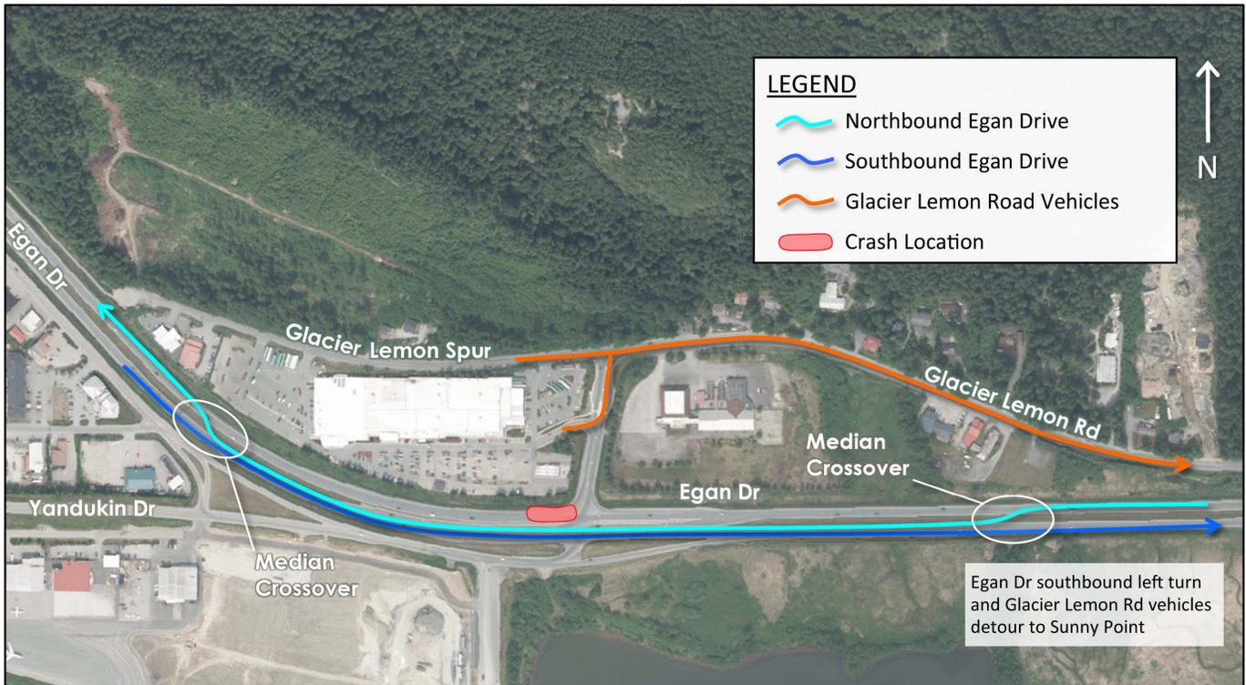
**Figure 11: Detour Route under Median Crossover Element After Median Crossover Traffic Control is Set Up**
