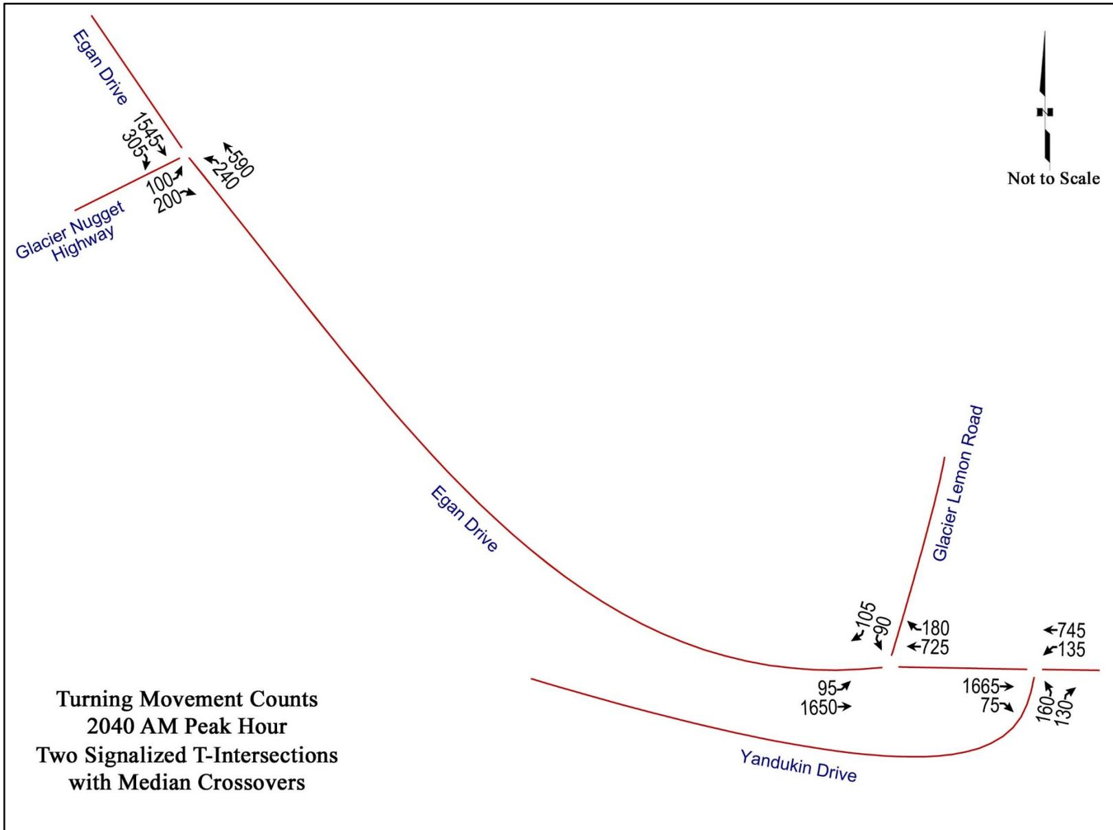
Figure D-9: Turning Movement Volumes – Two Signalized T-Intersections with Median Crossovers, 2040 AM Peak
