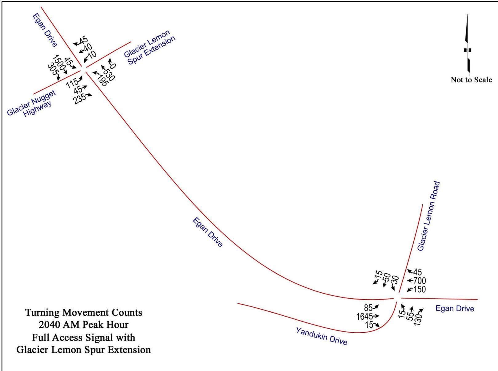
Figure D-7: Turning Movement Volumes – Full Access Signal with Glacier Lemon Spur Extension, 2040 AM Peak
