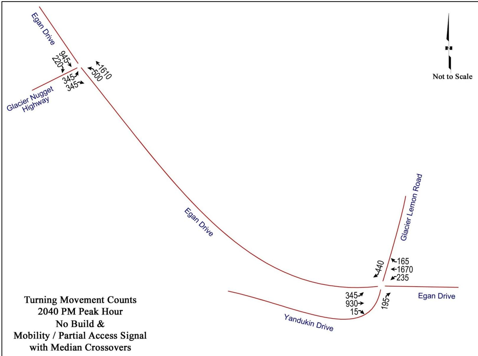
Figure D-2: Turning Movement Volumes – No Build, Mobility, and Partial Access Signal with Median Crossovers, 2040 PM Peak
