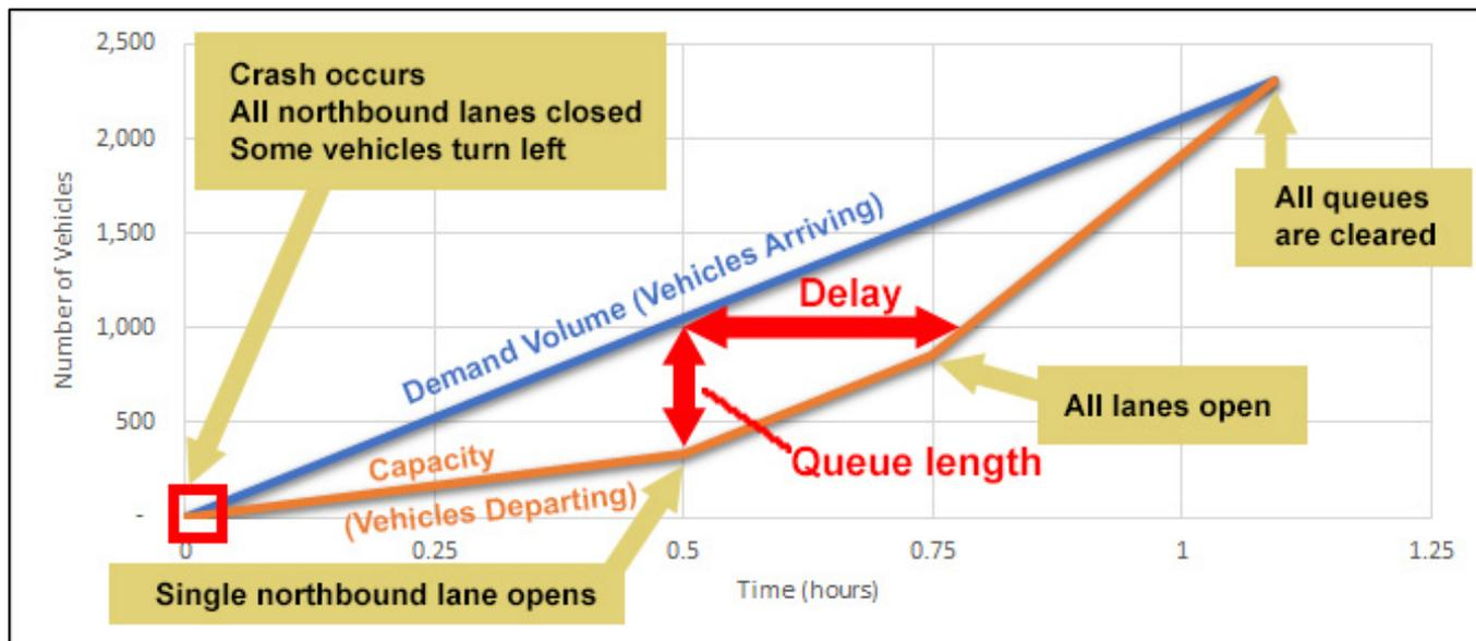
**Figure 10: Demand-Capacity Curve for No Build Alternative in 2040, Northbound PM Peak**
