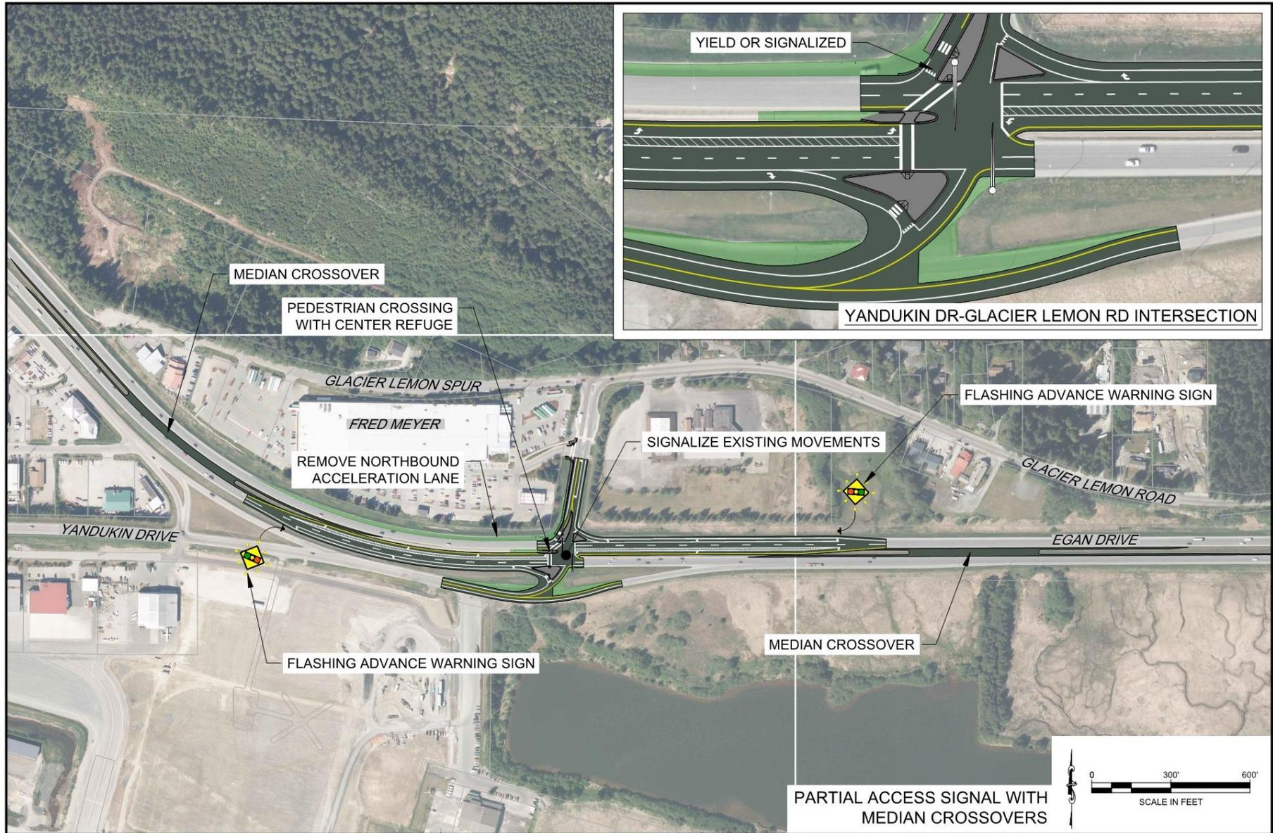
Figure 3: Partial Access Signal Concept Design
