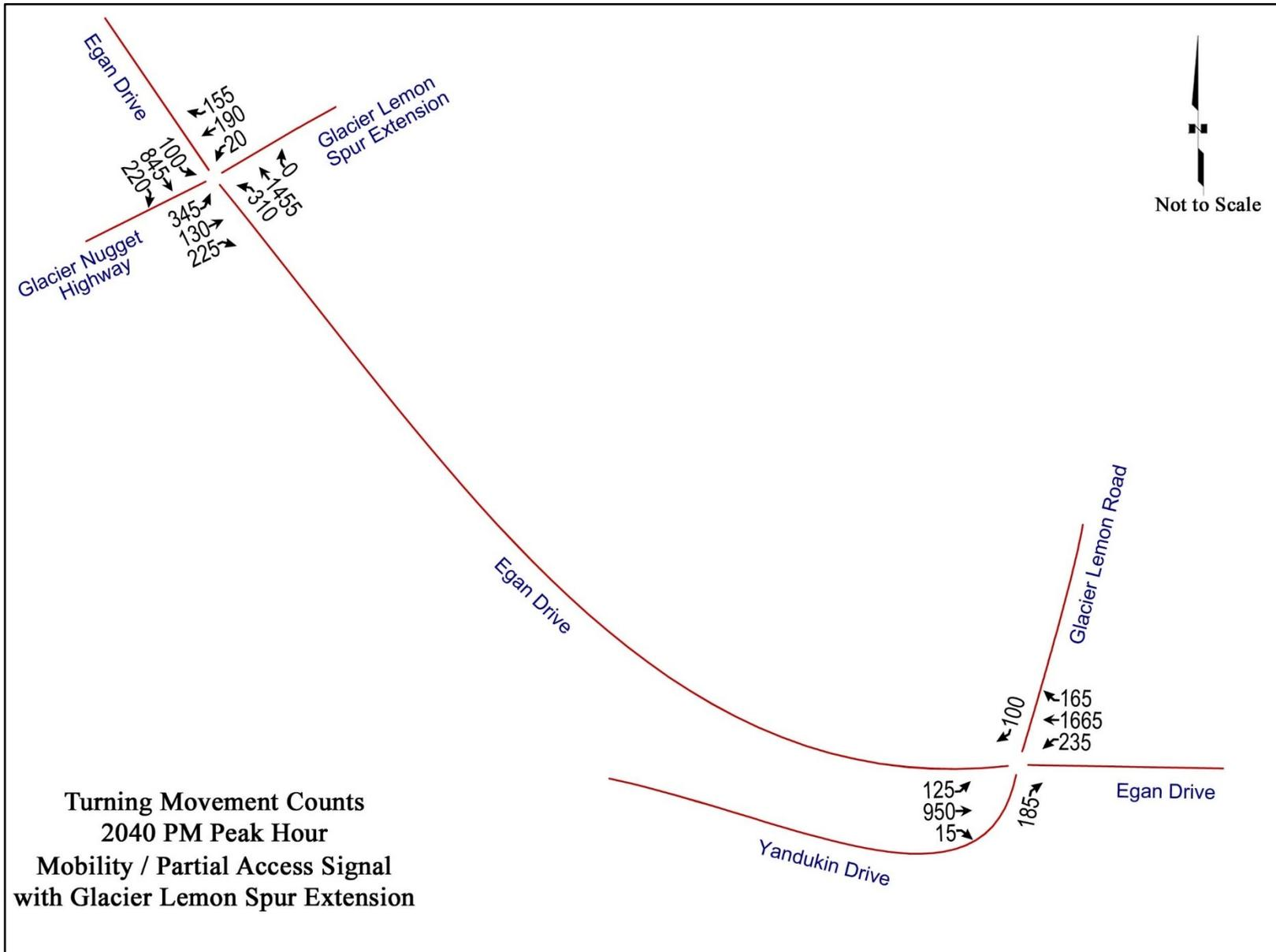
Figure D-4: Turning Movement Volumes – Mobility and Partial Access Signal with Glacier Lemon Spur Extension, 2040 PM Peak
