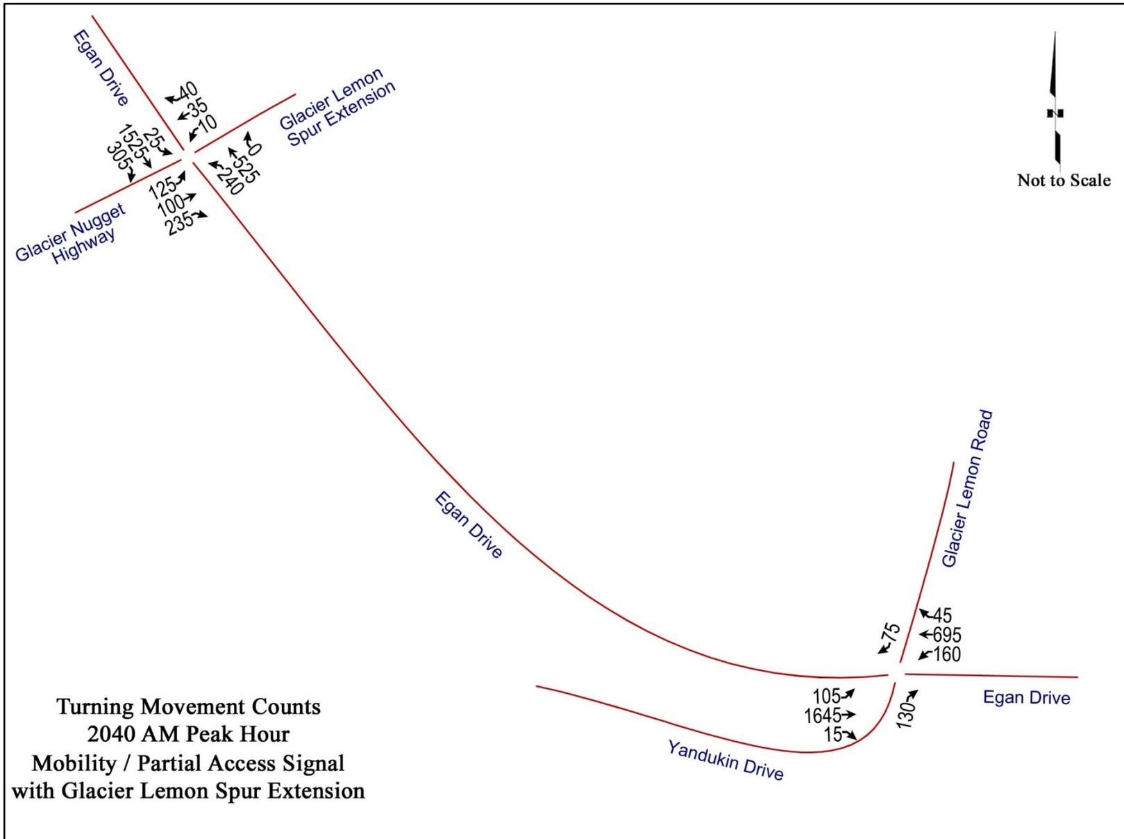
Figure D-3: Turning Movement Volumes – Mobility and Partial Access Signal with Glacier Lemon Spur Extension, 2040 AM Peak
