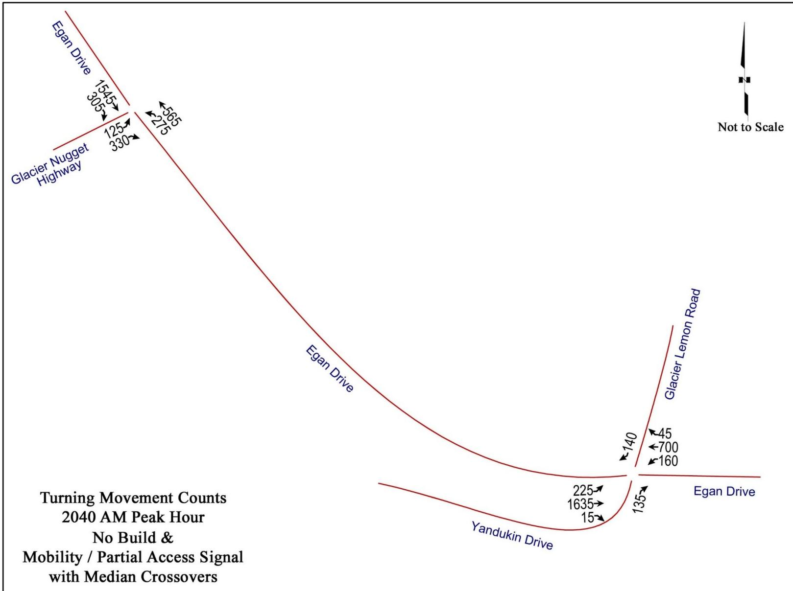
Figure D-1: Turning Movement Volumes – No Build, Mobility, and Partial Access Signal with Median Crossovers, 2040 AM Peak
