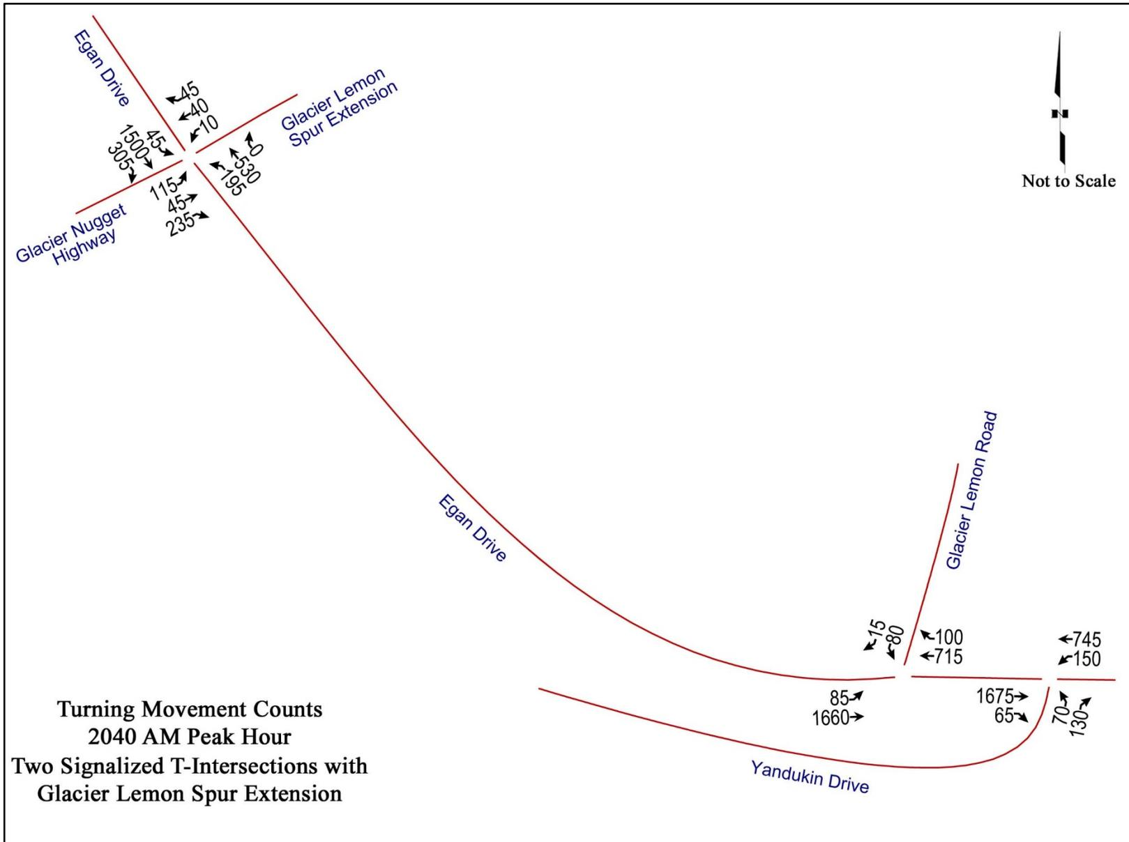
Figure D-11: Turning Movement Volumes – Two Signalized T-Intersections with Glacier Lemon Spur Extension, 2040 AM Peak
