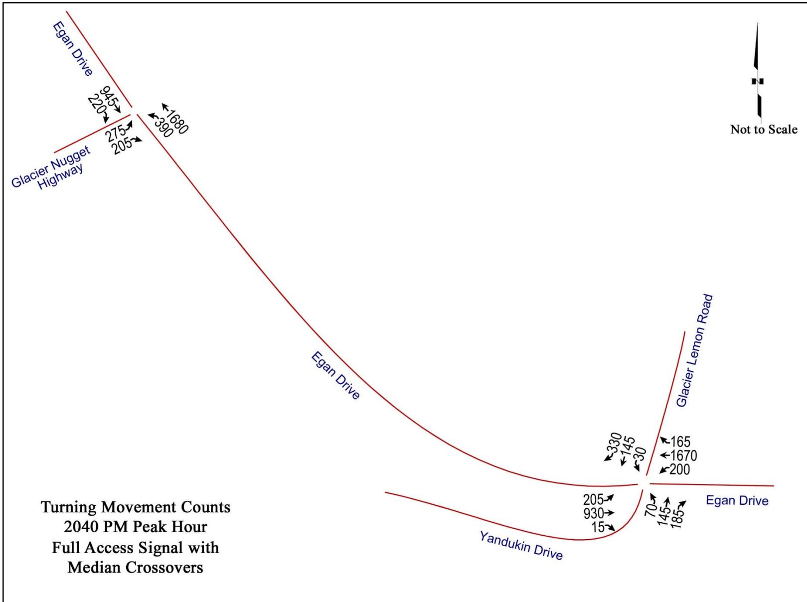
Figure D-6: Turning Movement Volumes – Full Access Signal with Median Crossovers, 2040 PM Peak
