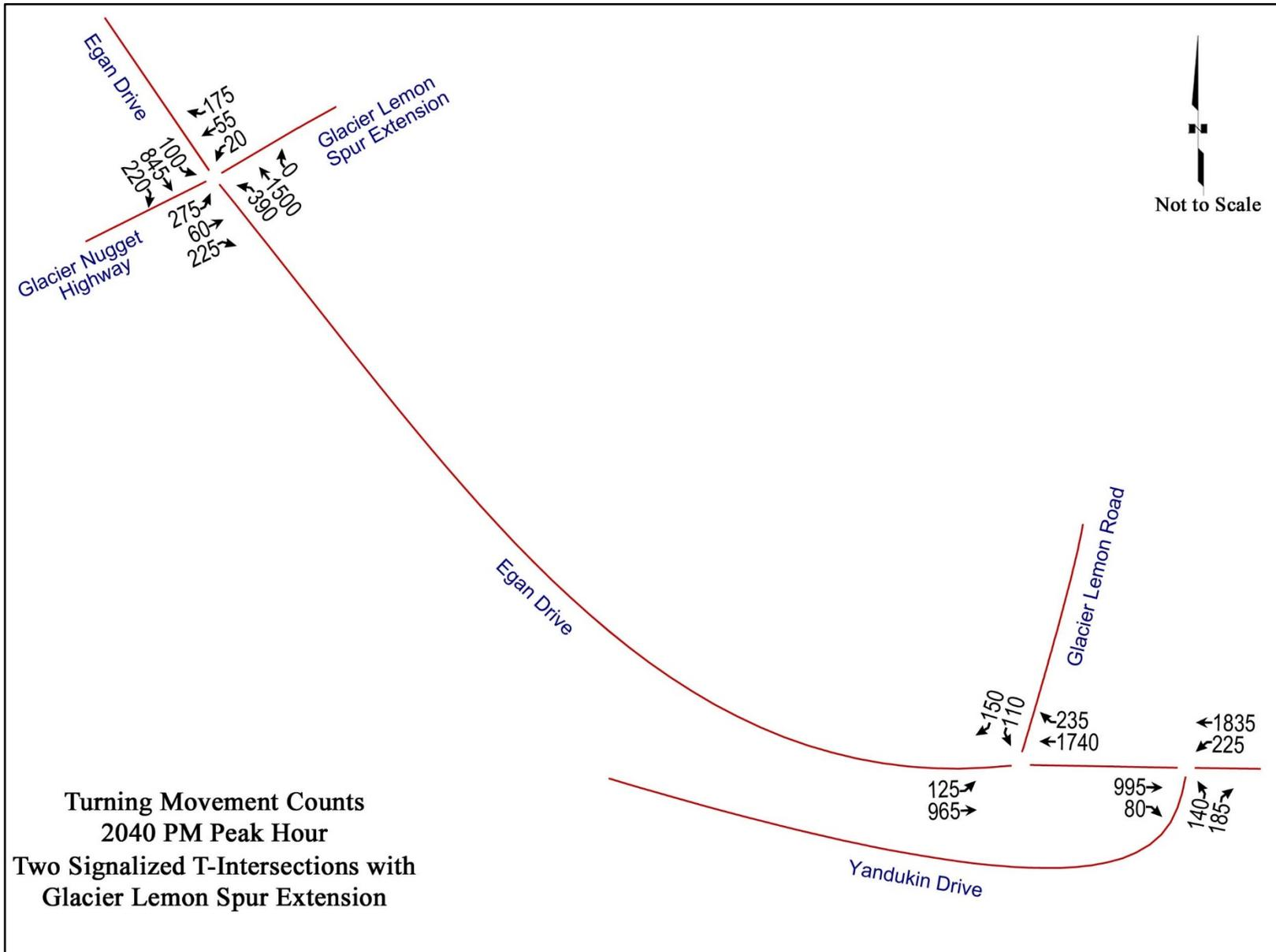
Figure D-12: Turning Movement Volumes – Two Signalized T-Intersections with Glacier Lemon Spur Extension, 2040 PM Peak
