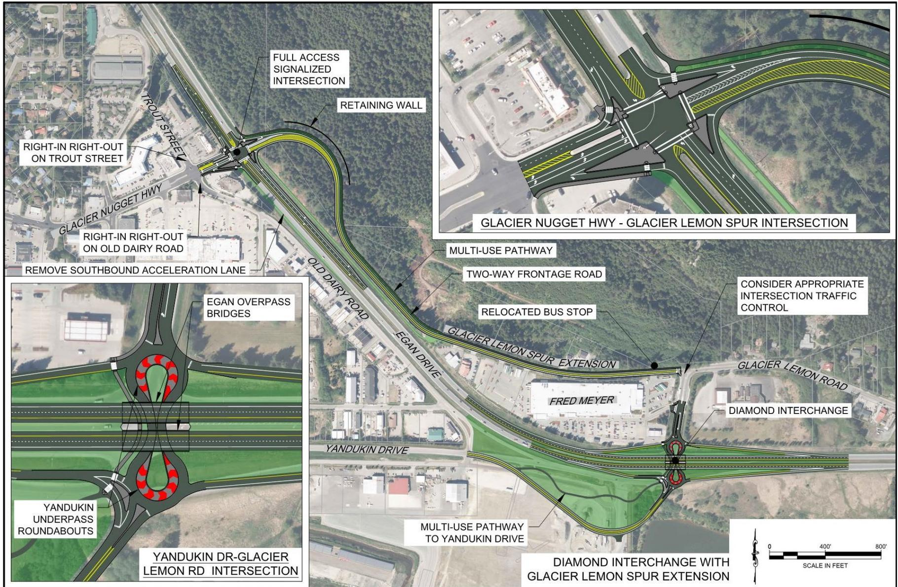
Figure 6: Diamond Interchange Concept Design
