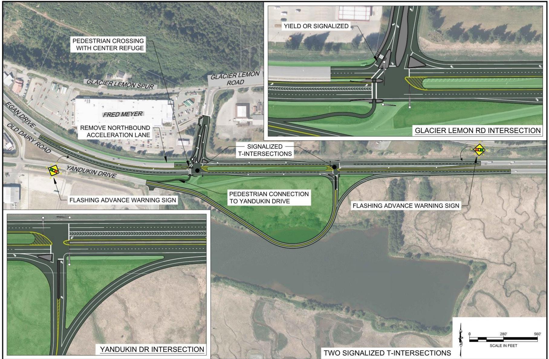
Figure 5: Two Signaled T-Intersections Concept Design
