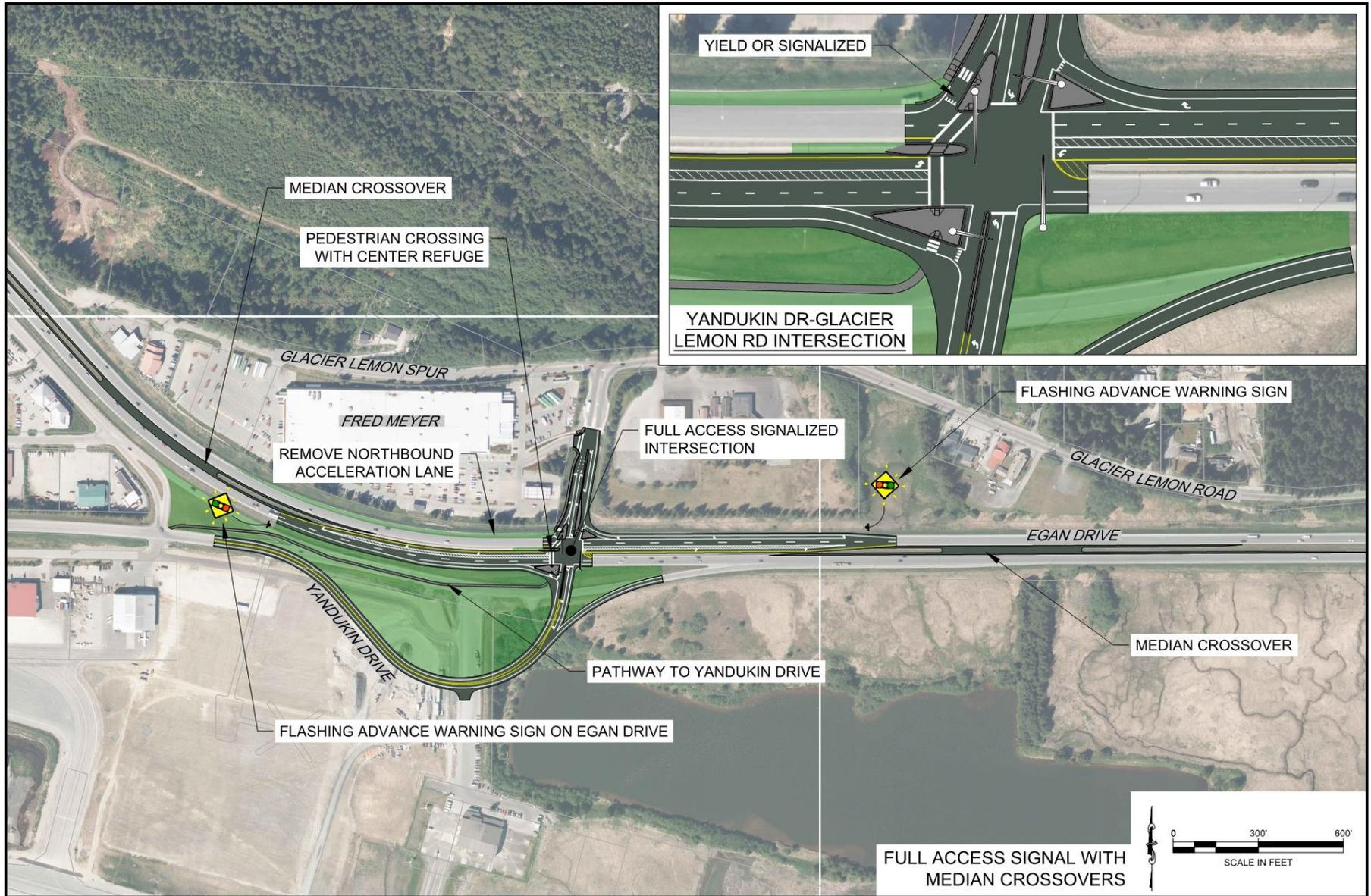
Figure 4: Full Access Signal Concept Design
