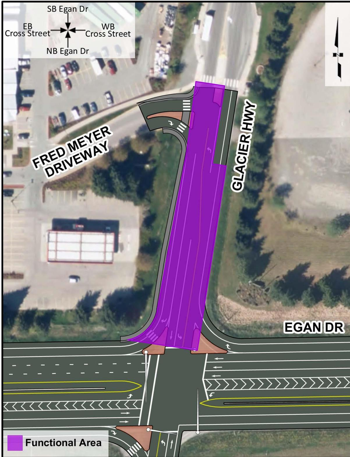
Figure 34. Functional Area, Alternative Concept B (Signal)
