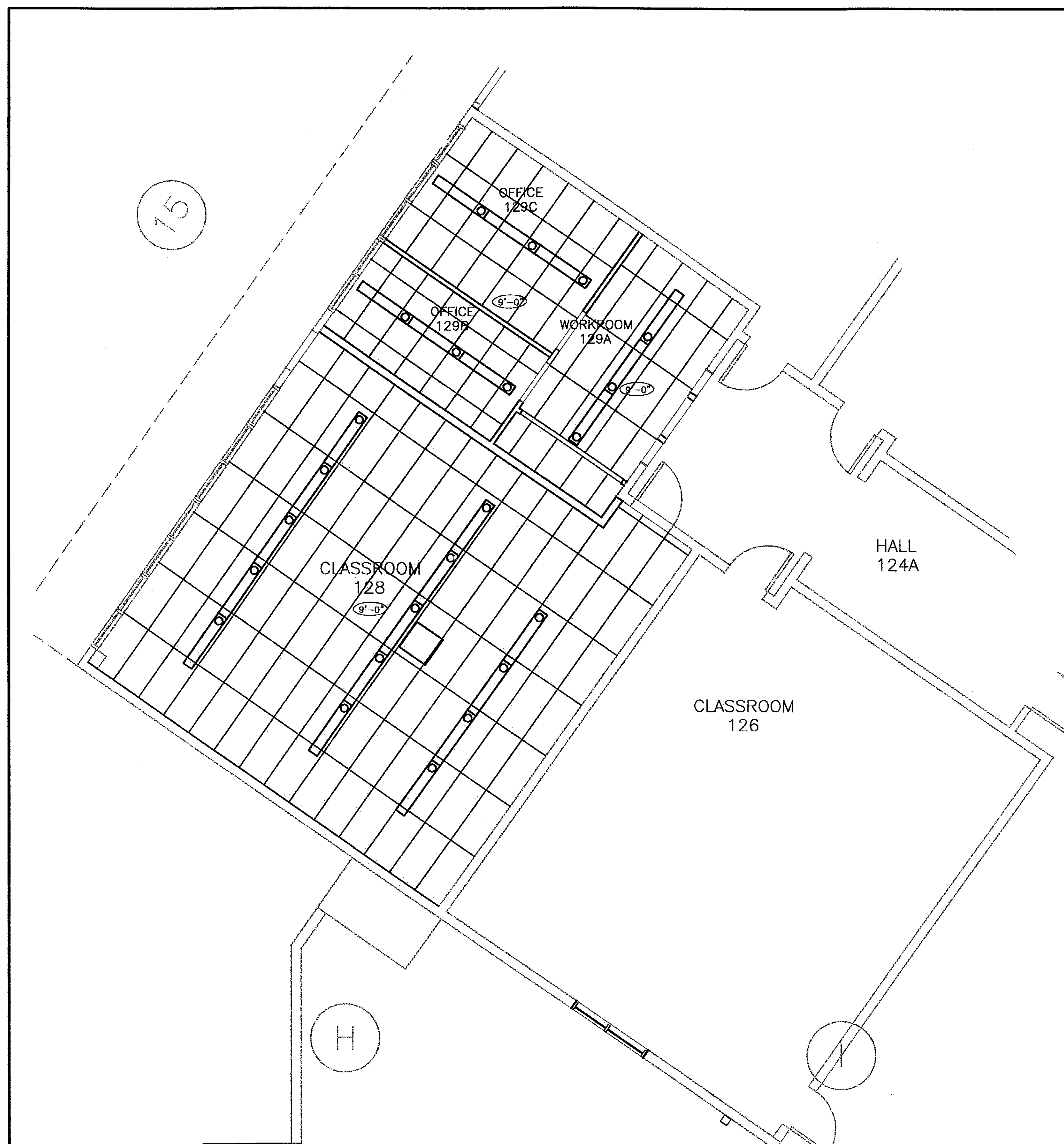
1 REFLECTED CEILING PLAN OFFICE 129 AND CLASSROOM 8 SCALE: 0 2' 4' 8'
