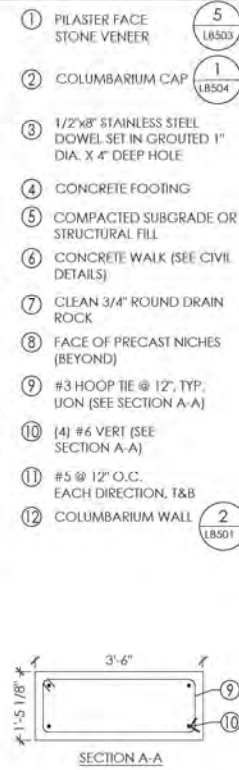
2 COLUMBARIUM - PILASTER END SECTION - 5 HIGH
