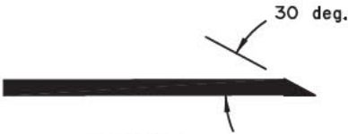
FIGURE 4 Safety Edge Detail
