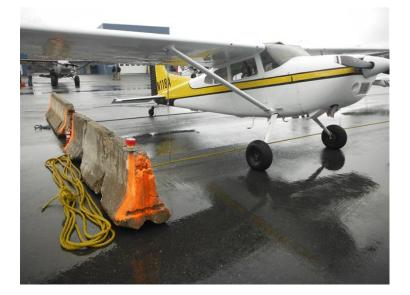
An alternative tie down system that allows cables to be anchored to an embedded engineered system would be beneficial. This alternative would remove the Jersey Barrier hazard to taxiing aircraft.
