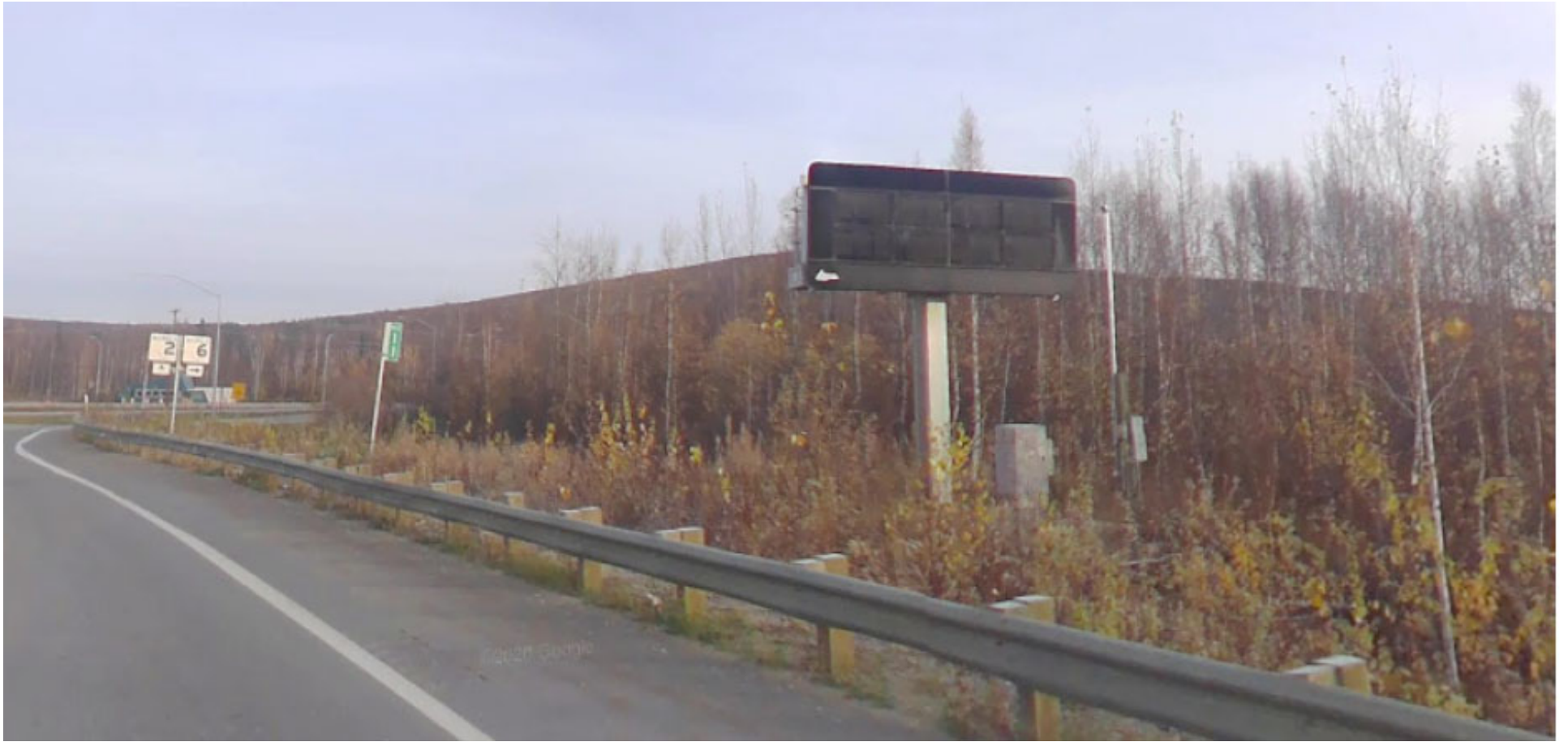
Photo Example of Dynamic Messaging Sign (DMS)
