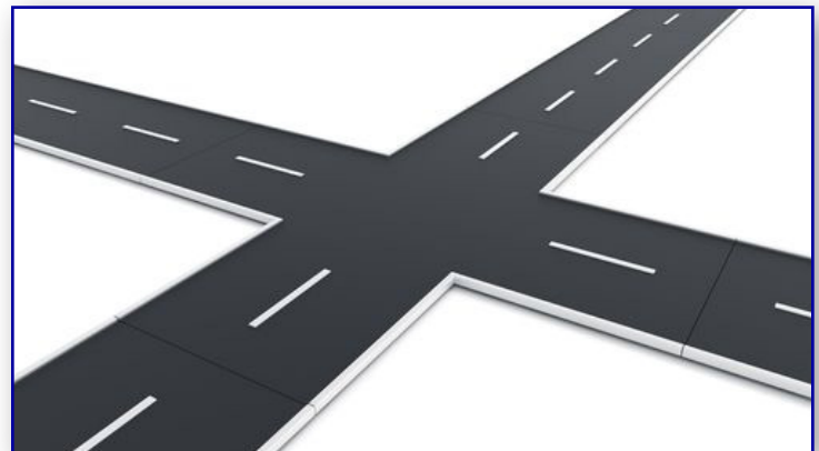
An at-grade intersection joins two or more roads and can include traffic signals, stop signs, or yield signs.
