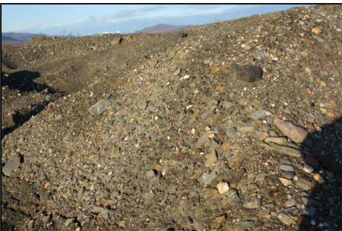
Photo 33: Typical stockpile of material, displaying possible cobble and boulder content of till.
