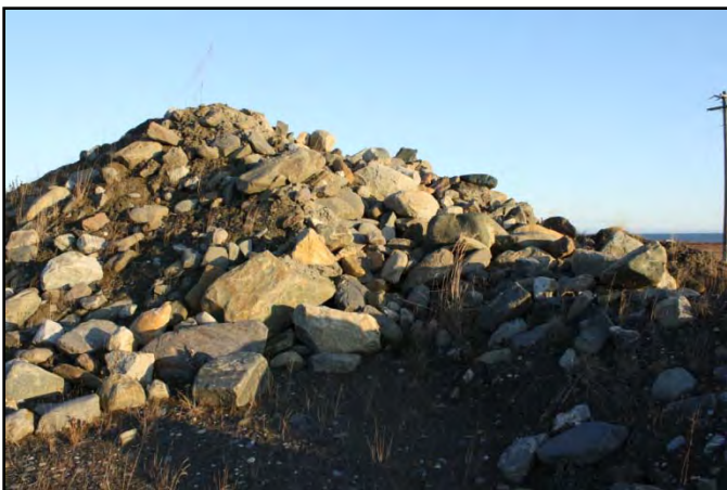
Photo 39: Typical stockpile of material, displaying possible cobble and boulder content of till.
