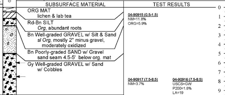
Drilling Notes: Test Trench dug with a Case 1150 C Backhoe. Trench dimensions were 16' long x 2.5' wide
