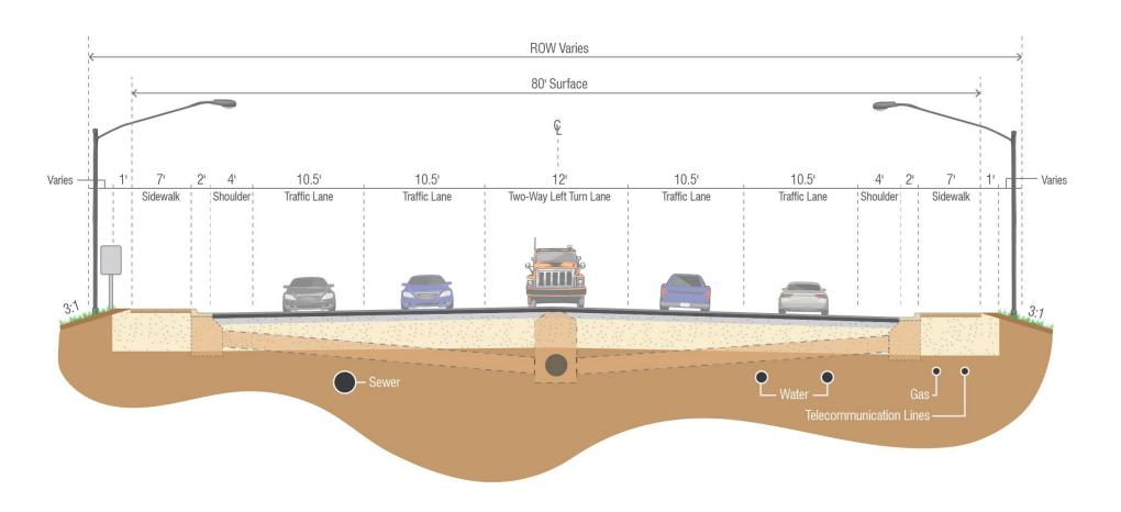
**Figure 3: Typical Section Stage 1**
