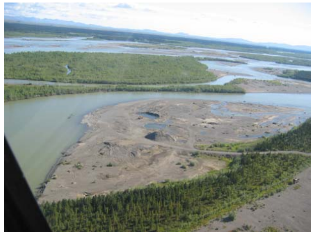
Figure 8 – Aerial photo of point bar currently used as material source.
