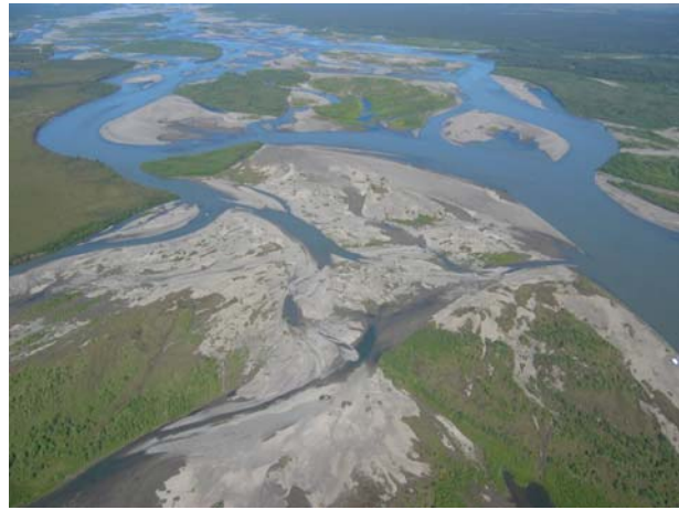
Figure 10 – Looking upriver at island. Note severe deflection of main channel at head of island.
