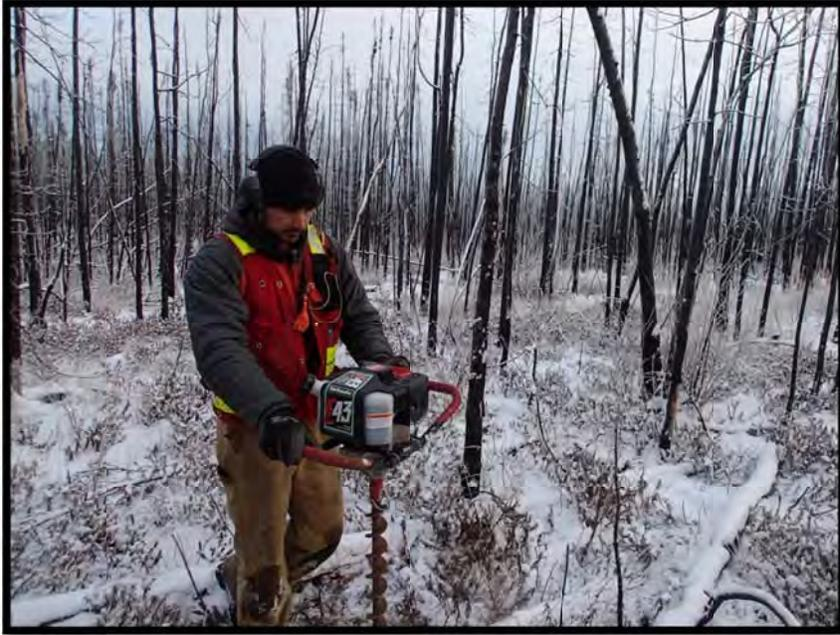
*Photo 0097 – gas-powered auger used for geotechnical sampling*
