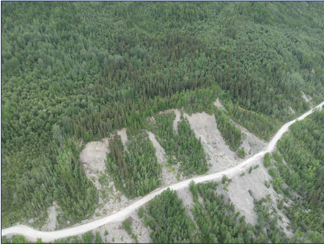
Figure 1-8. Examples of Landslide Areas near MP 58 and Kotsina Bluffs
