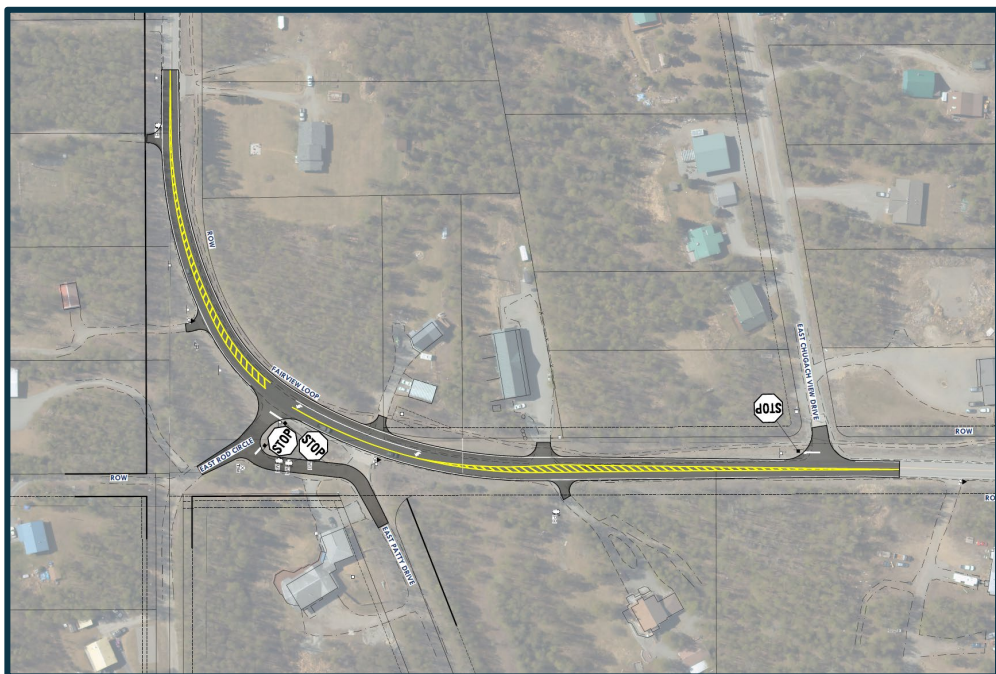
H2 - Existing Alignment – Single Approach – Left Turn Pocket
